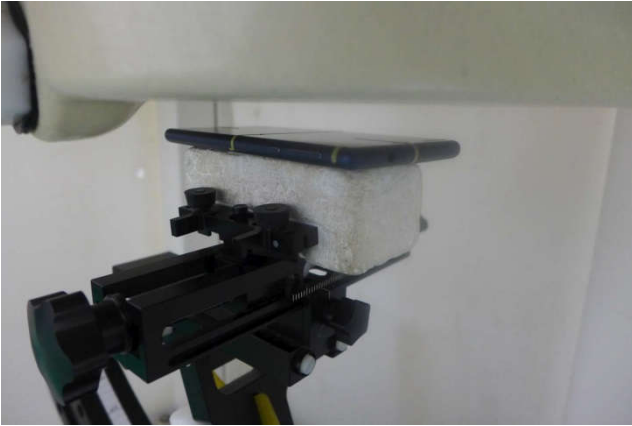
Front, Test Separation 15 mm
