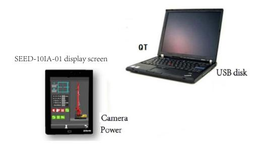
The configuration development software QT is installed on the PC. The power supply and camera are connected to the display screen, and the platform is built.
