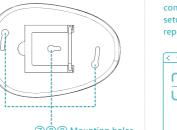
The hole in center is for wall-mounting. the other two are for ceiling-mounting
