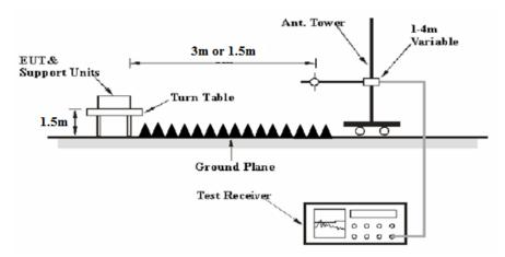
Note: for 18GHz-40GHz and Band edge test was at 1.5m distance, for other emissions test was at 3m distance.
