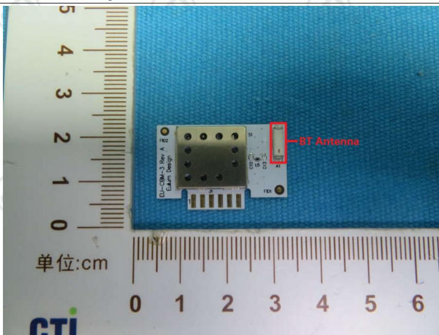
The antenna is chip Antenna and no consideration of replacement. The best case gain of the antenna is 1.3dBi.
