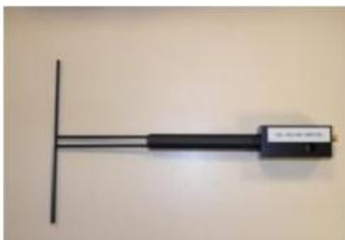
Figure 1 – Satimo COMOSAR Validation Dipole
