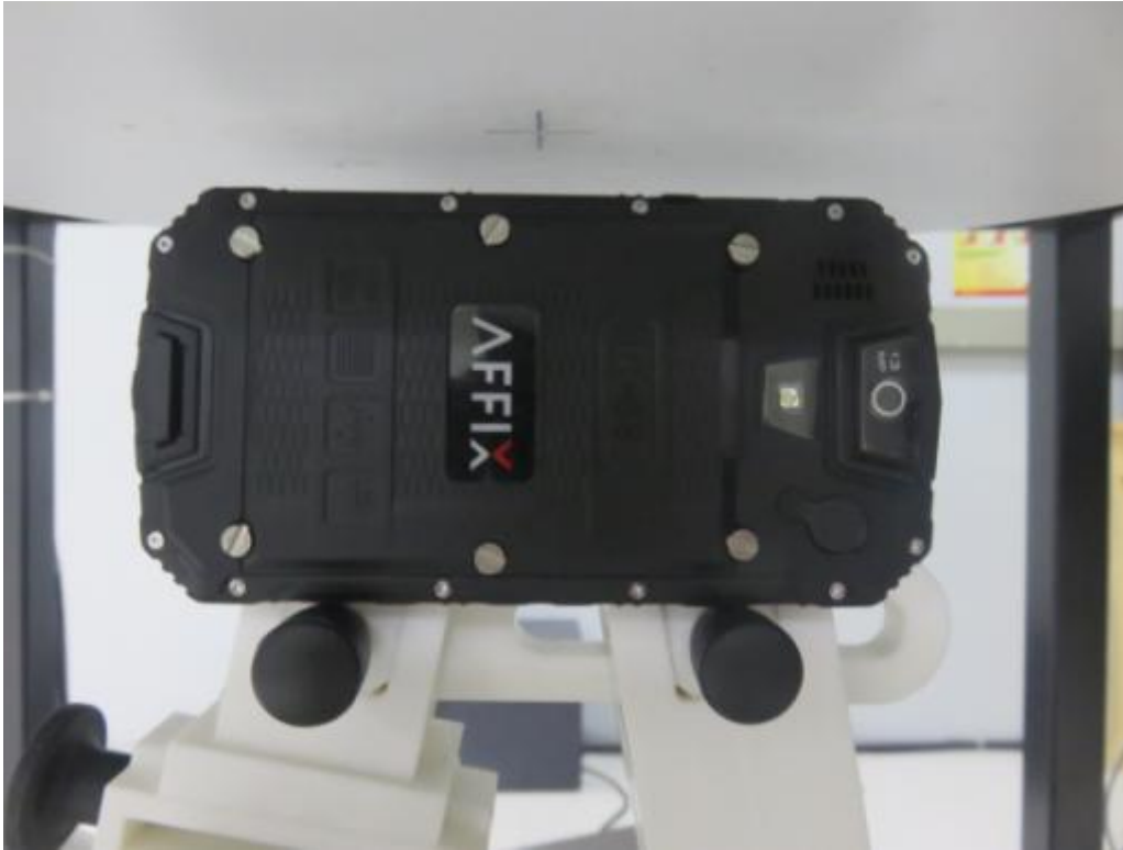
10mm body-worn Right Side Setup Photo(hotspot)
