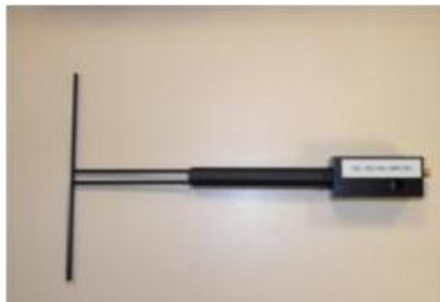
Figure 1 – Satimo COMOSAR Validation Dipole
