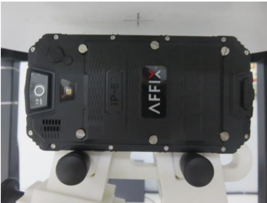
10mm body-worn Left Side Setup Photo(hotspot)
