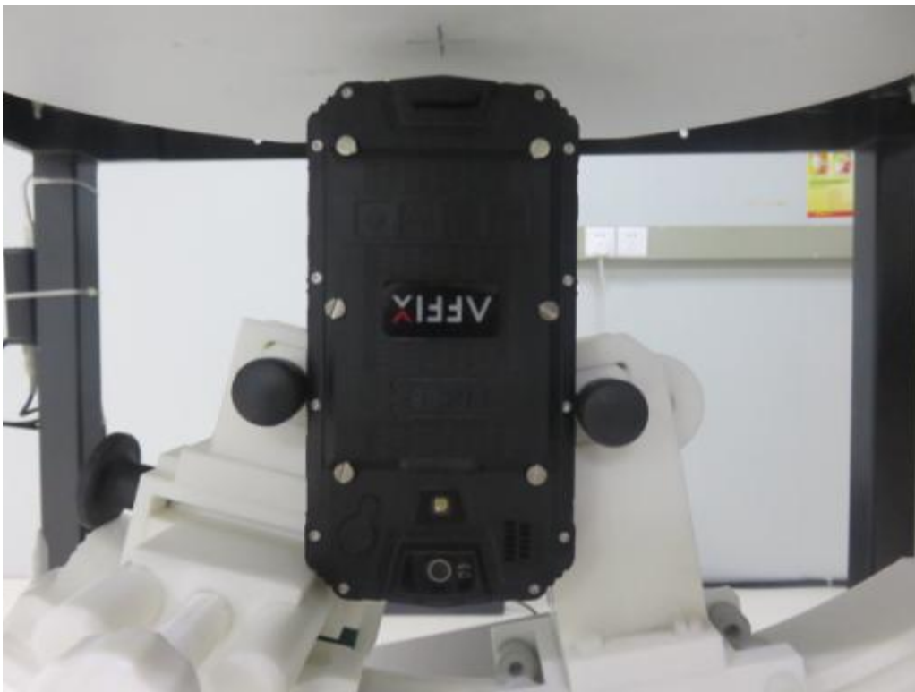
10mm body-worn Bottom Side Setup Photo(hotspot)
