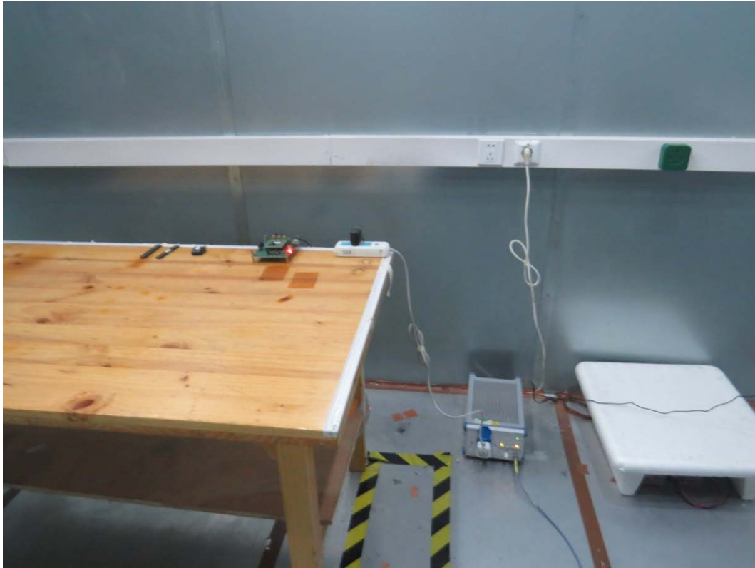
Picture 3 Conducted Emission Test Setup
