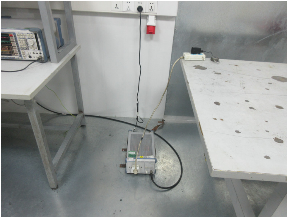
Photo of Power Line Conducted Emission Test
