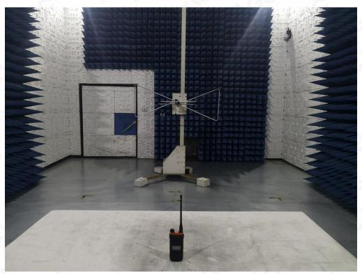
RADIATED EMISSION ABOVE 1G TEST SETUP
