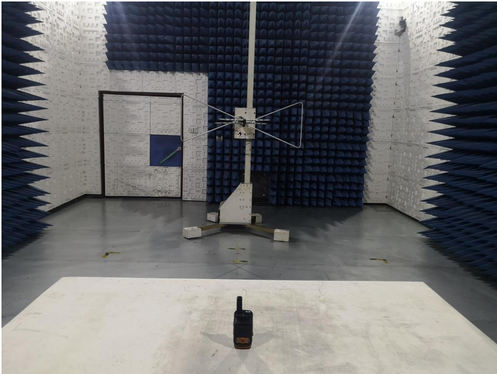
RADIATED EMISSION ABOVE 1G TEST SETUP
