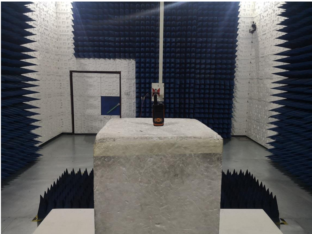
RADIATED EMISSION ABOVE 1G TEST SETUP
