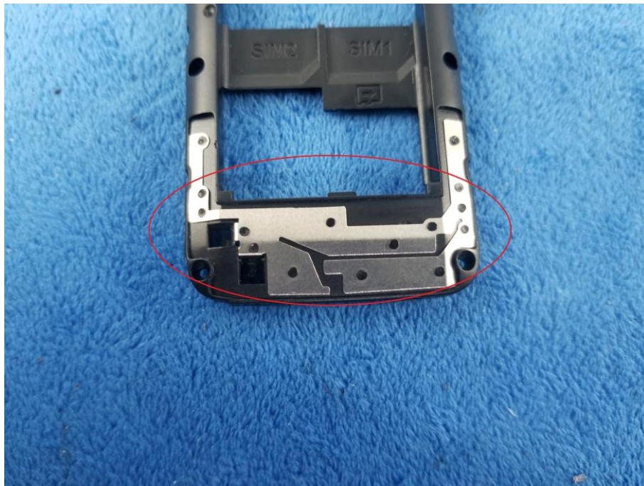
GSM/PCS - Antenna View
