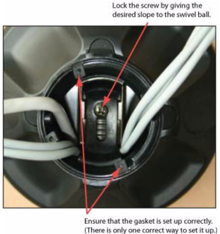
Figure 17 Routing the cables into the swivel
