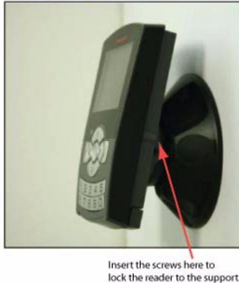
Figure 19 Locking the reader onto the swivel support
