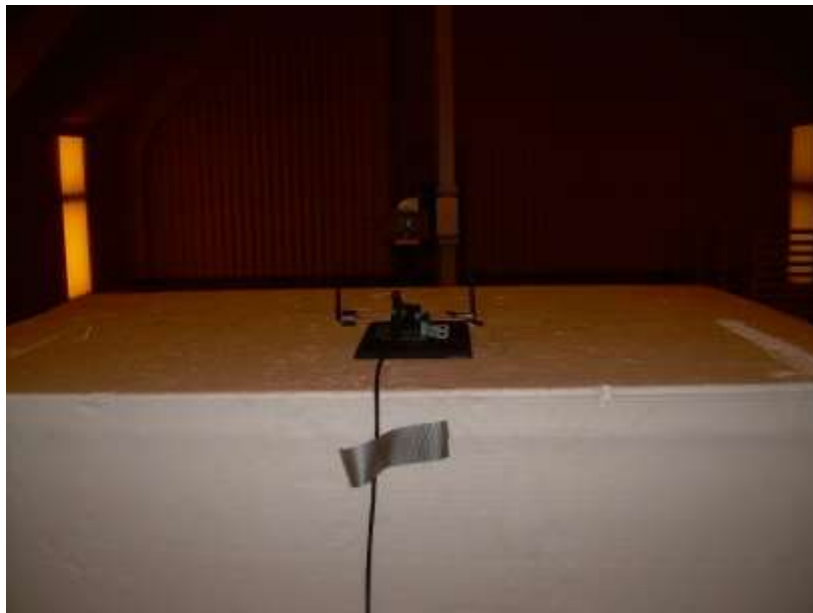
Photograph 4: Back View Radiated Emissions Worst-Case Configuration (Module Flat and Antennas Vertical) – Above 1000 MHz
