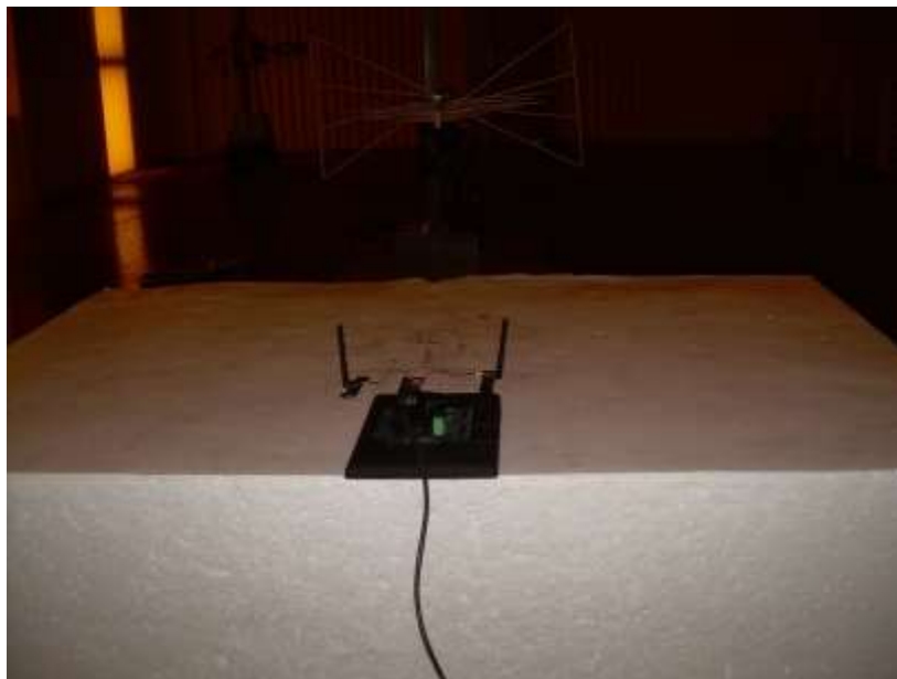
Photograph 2: Back View Radiated Emissions Worst-Case Configuration
