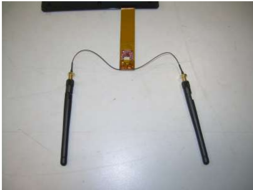
Photograph 7: View Radiated Emissions Module Flat and Antennas Flat
