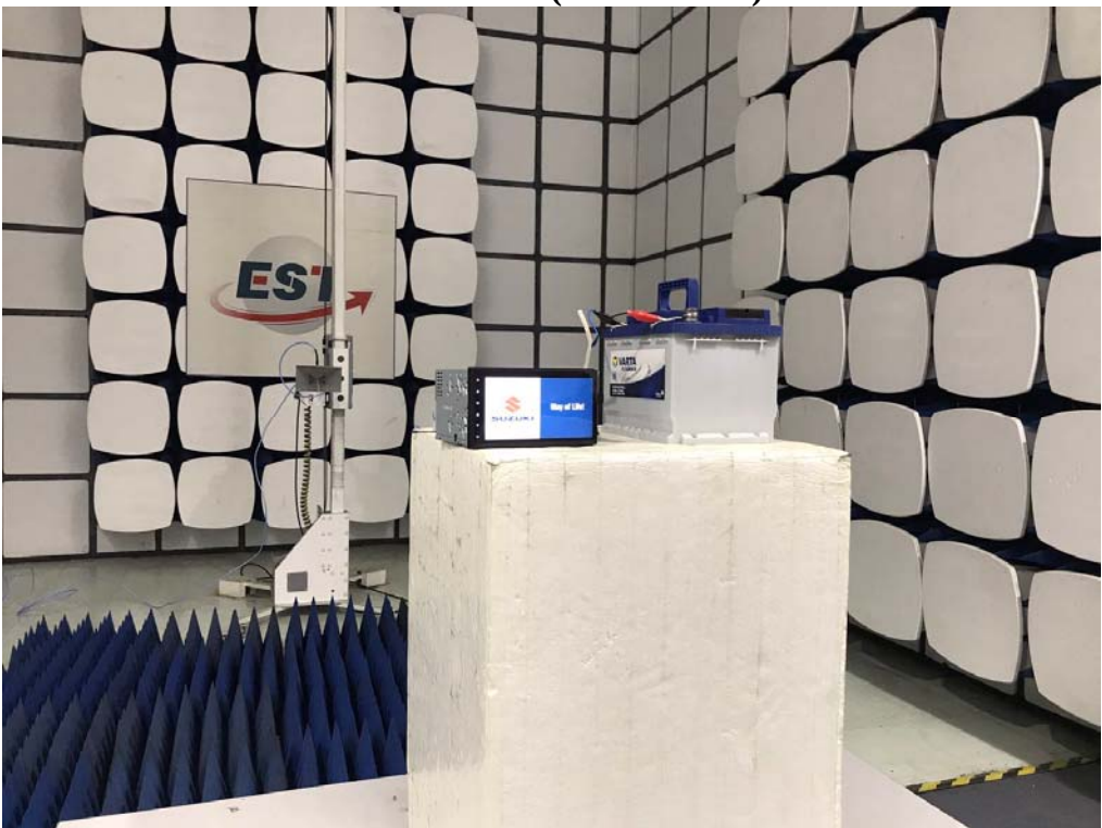
Radiated Test (Above 1GHz)
