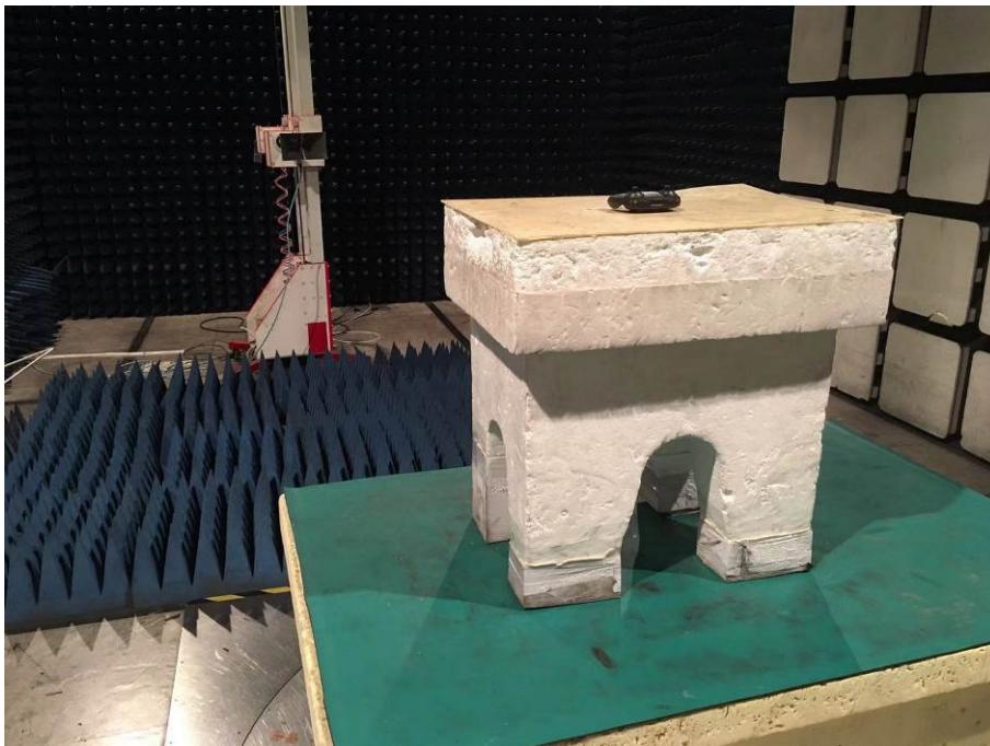
Spurious Emission Test Setup (Above 1GHz)
