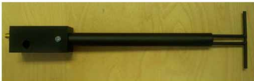
Figure 1 – MVG COMOSAR Validation Dipole
