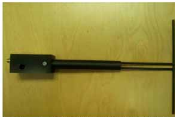
Figure 1 – MVG COMOSAR Validation Dipole
