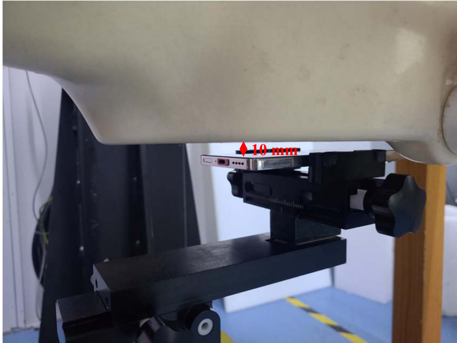
Body (Worn) Front Setup Photo (10mm)
