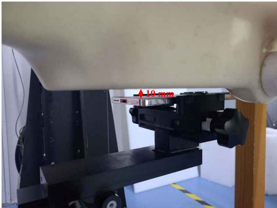
Body (Worn) Back Setup Photo (10mm)
