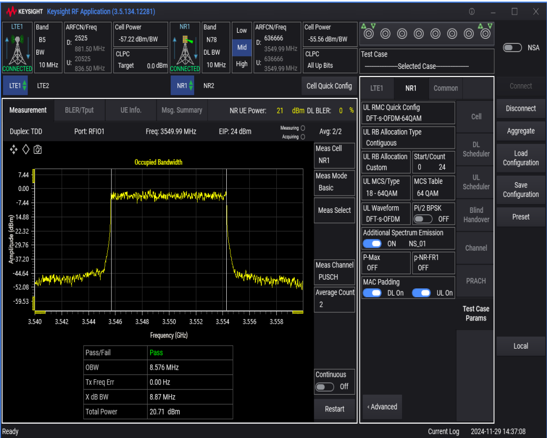
n78 SCS=30kHz DFT_QAM256 BW=90MHz Channel=636666 RB=240@0
