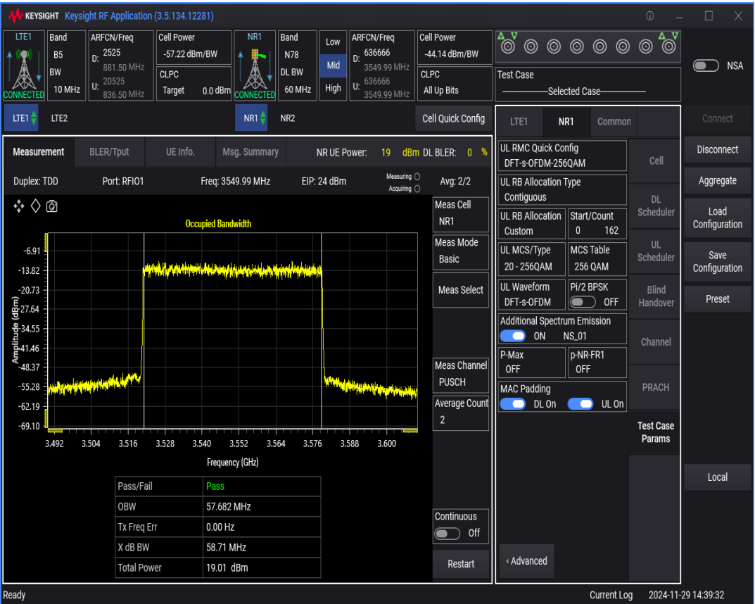
n78 SCS=30kHz DFT_QAM256 BW=80MHz Channel=636666 RB=216@0
