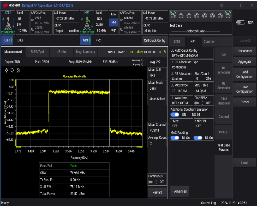
n78 SCS=30kHz DFT_QAM16 BW=90MHz Channel=636666 RB=240@0
