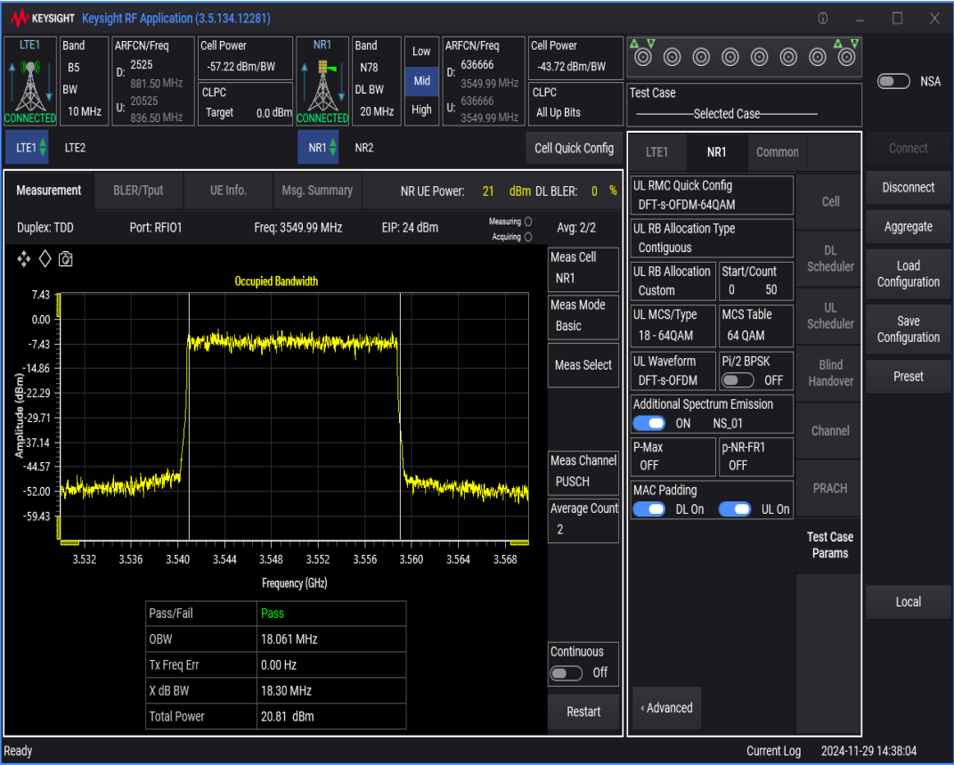
n78 SCS=30kHz DFT_QAM64 BW=15MHz Channel=636666 RB=36@0
