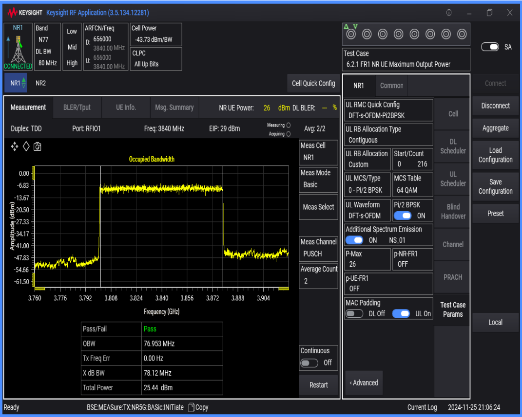
n77(3700-3980) SCS=30kHz DFT_BPSK BW=60MHz Channel=656000 RB=162@0
