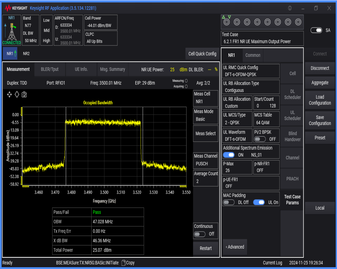
n77(3450-3550) SCS=30kHz DFT_QPSK BW=60MHz Channel=633334 RB=162@0
