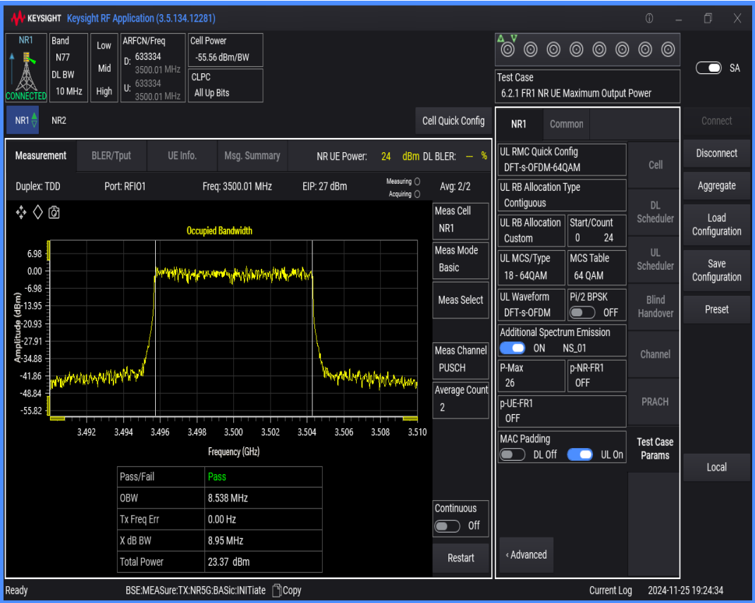
n77(3450-3550) SCS=30kHz DFT_QAM64 BW=15MHz Channel=633334 RB=36@0
