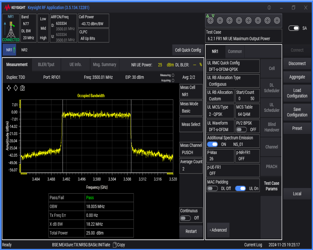
n77(3450-3550) SCS=30kHz DFT_QPSK BW=10MHz Channel=633334 RB=24@0
