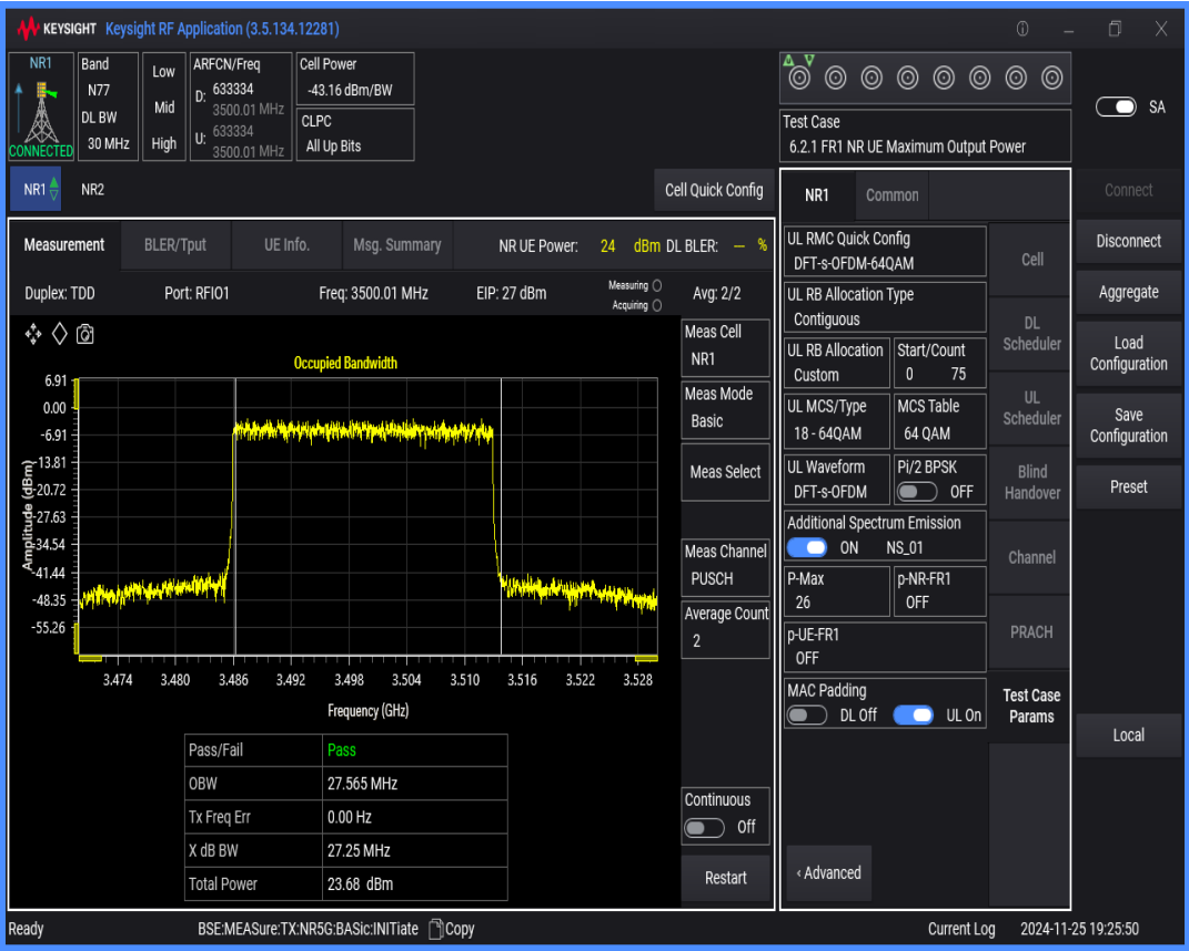
n77(3450-3550) SCS=30kHz DFT_QAM64 BW=10MHz Channel=633334 RB=24@0
