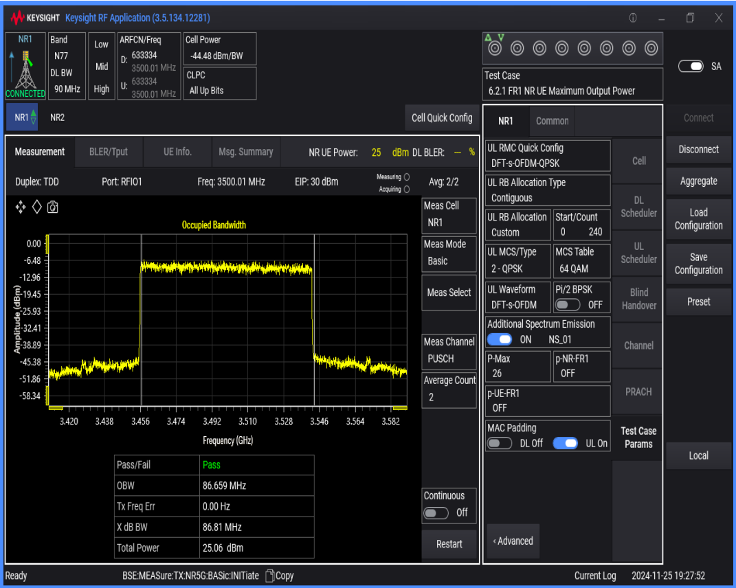
n77(3450-3550) SCS=30kHz DFT_QPSK BW=50MHz Channel=633334 RB=128@0
