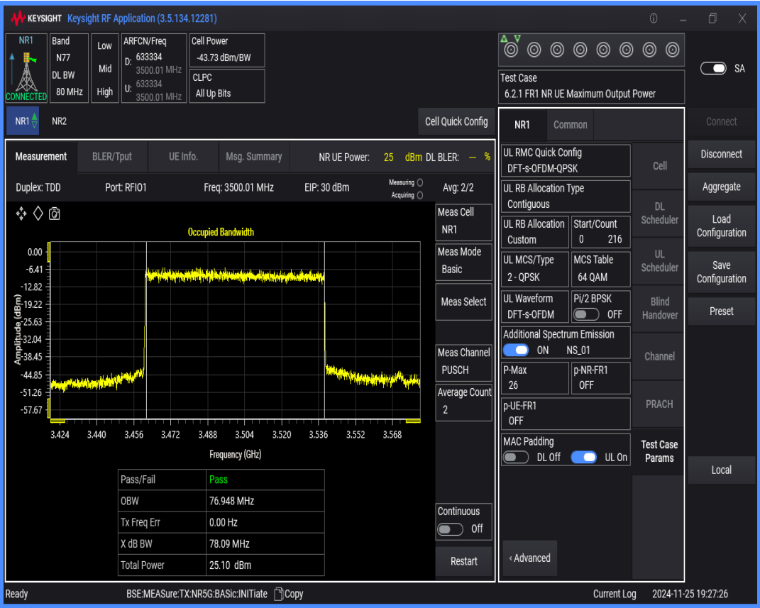
n77(3450-3550) SCS=30kHz DFT_QPSK BW=90MHz Channel=633334 RB=240@0
