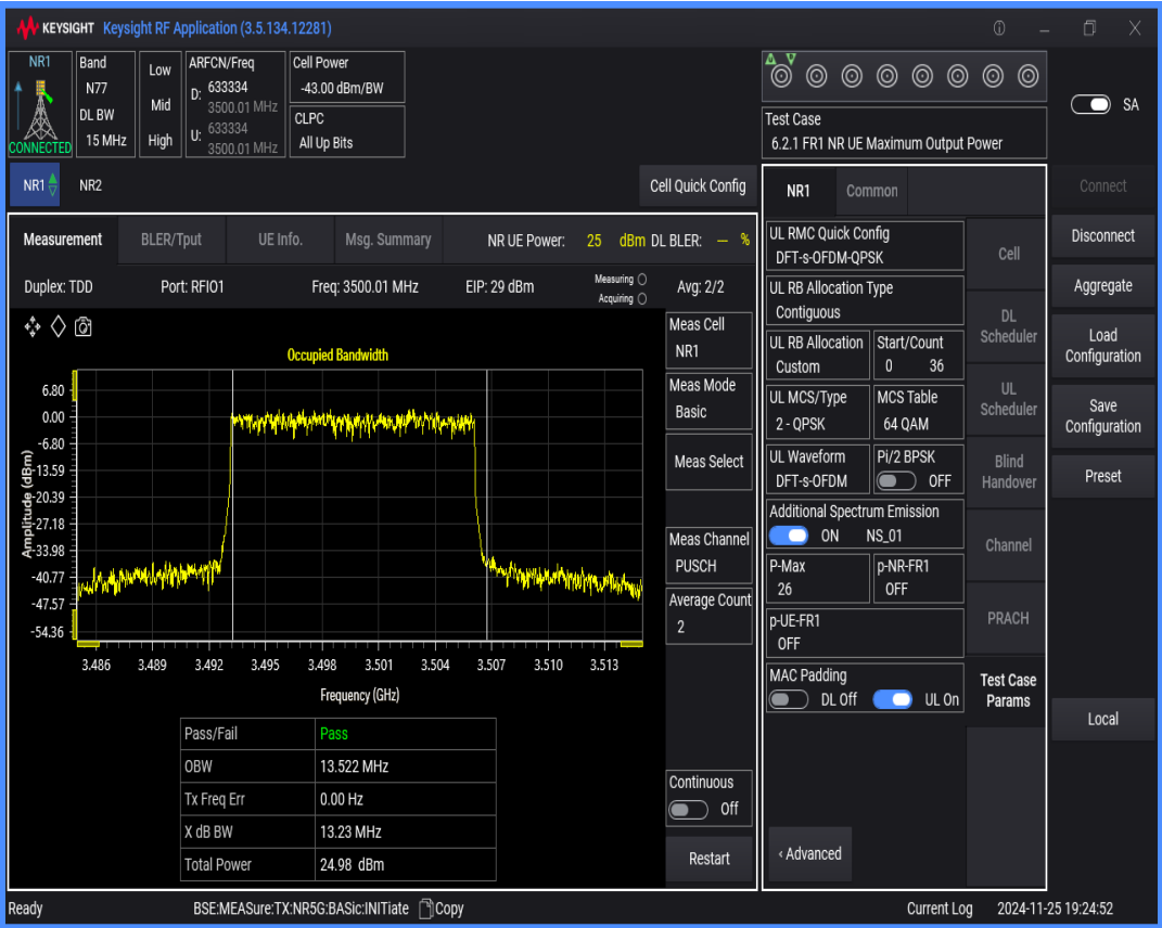
n77(3450-3550) SCS=30kHz DFT_QPSK BW=80MHz Channel=633334 RB=216@0
