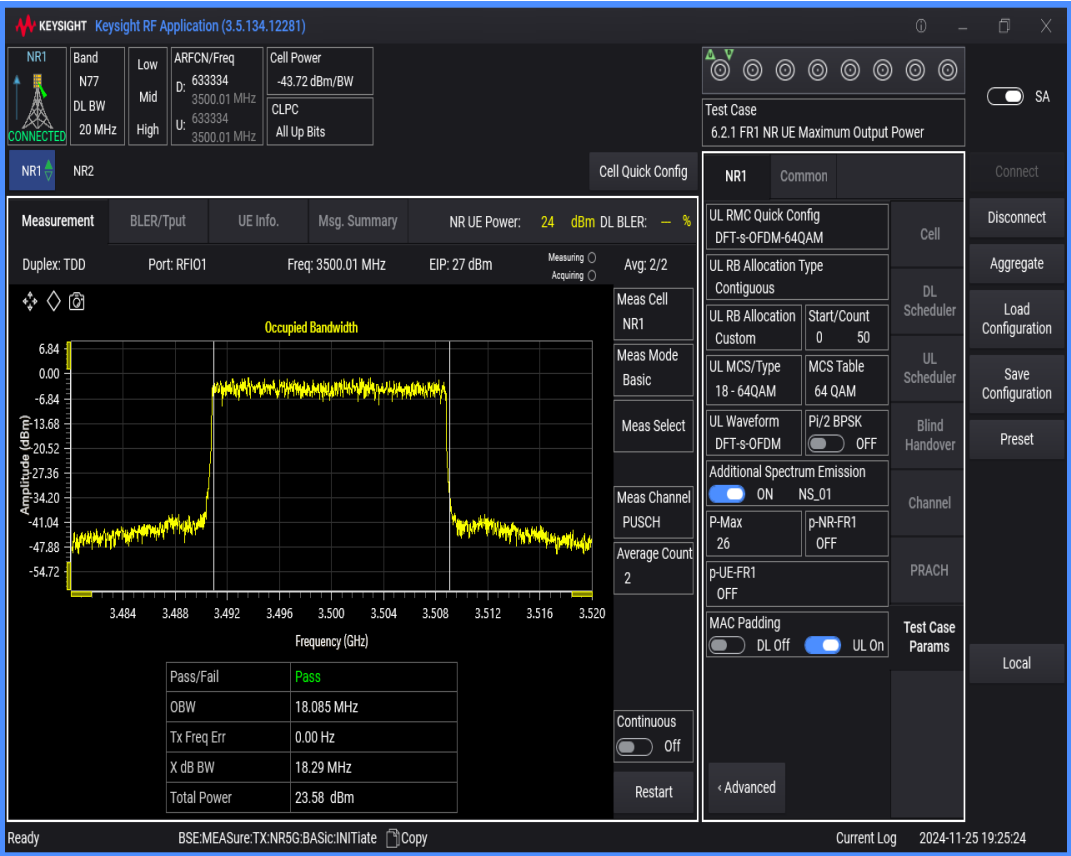
n77(3450-3550) SCS=30kHz DFT_QAM64 BW=30MHz Channel=633334 RB=75@0
