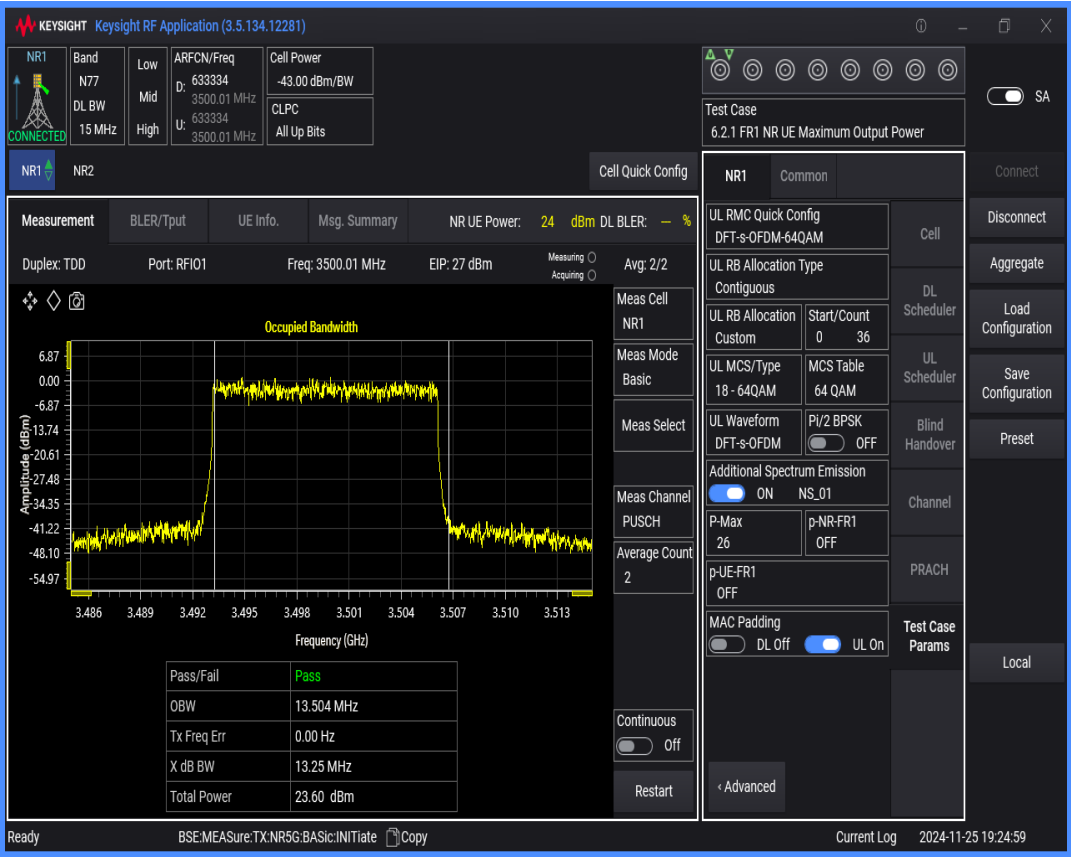
n77(3450-3550) SCS=30kHz DFT_QAM64 BW=80MHz Channel=633334 RB=216@0
