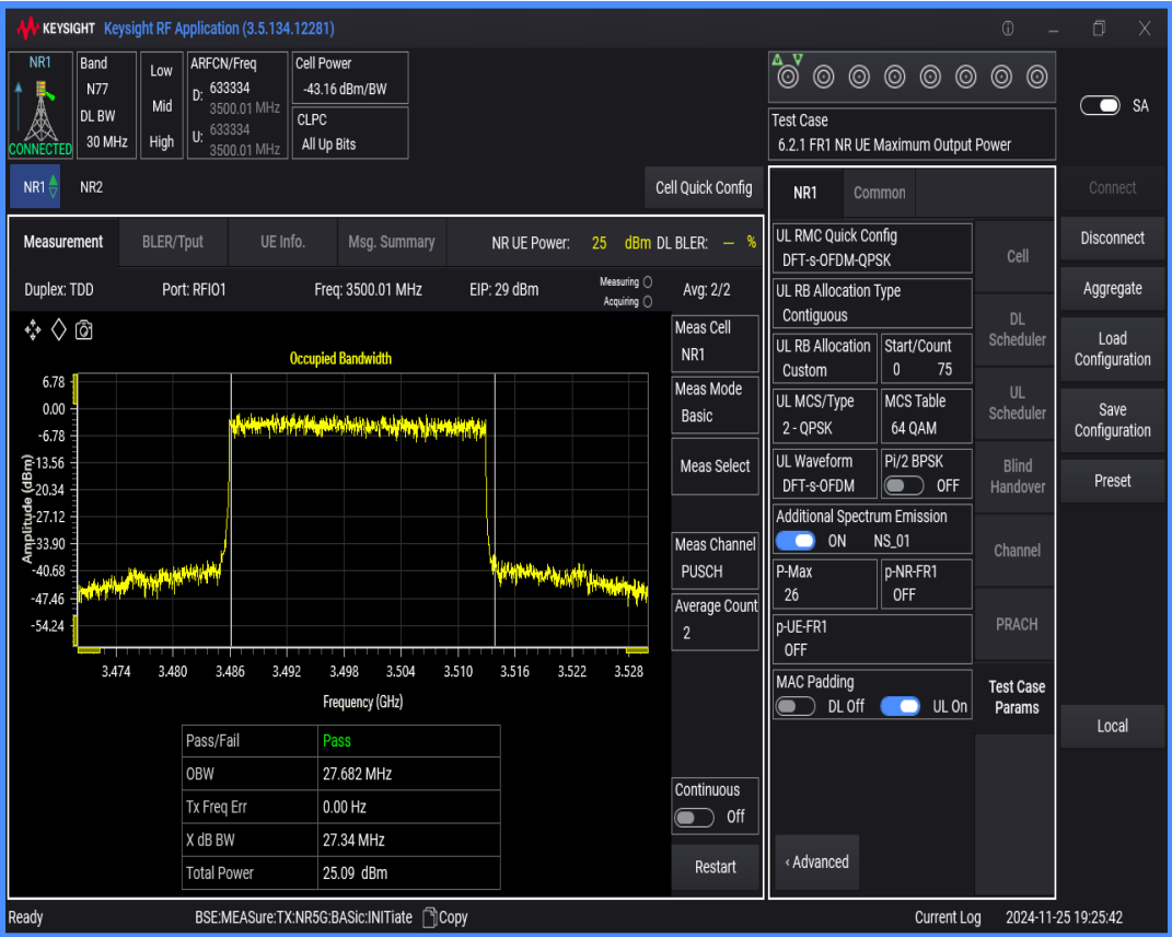
n77(3450-3550) SCS=30kHz DFT_QPSK BW=40MHz Channel=633334 RB=100@0
