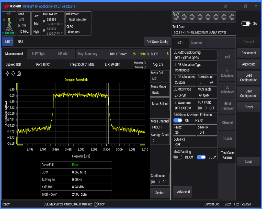
n77(3450-3550) SCS=30kHz DFT_QPSK BW=15MHz Channel=633334 RB=36@0
