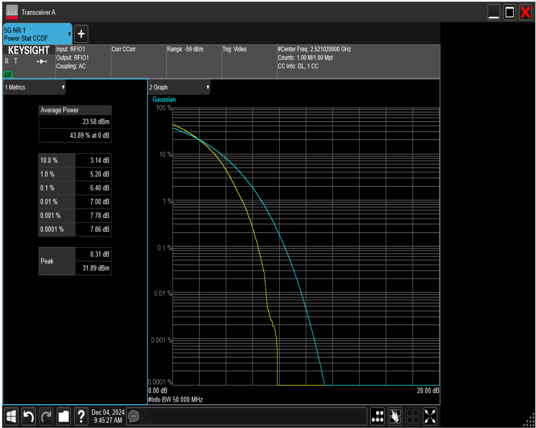
n41 SCS=30kHz DFT_QAM64 BW=50MHz Channel=518598 RB=128@0
