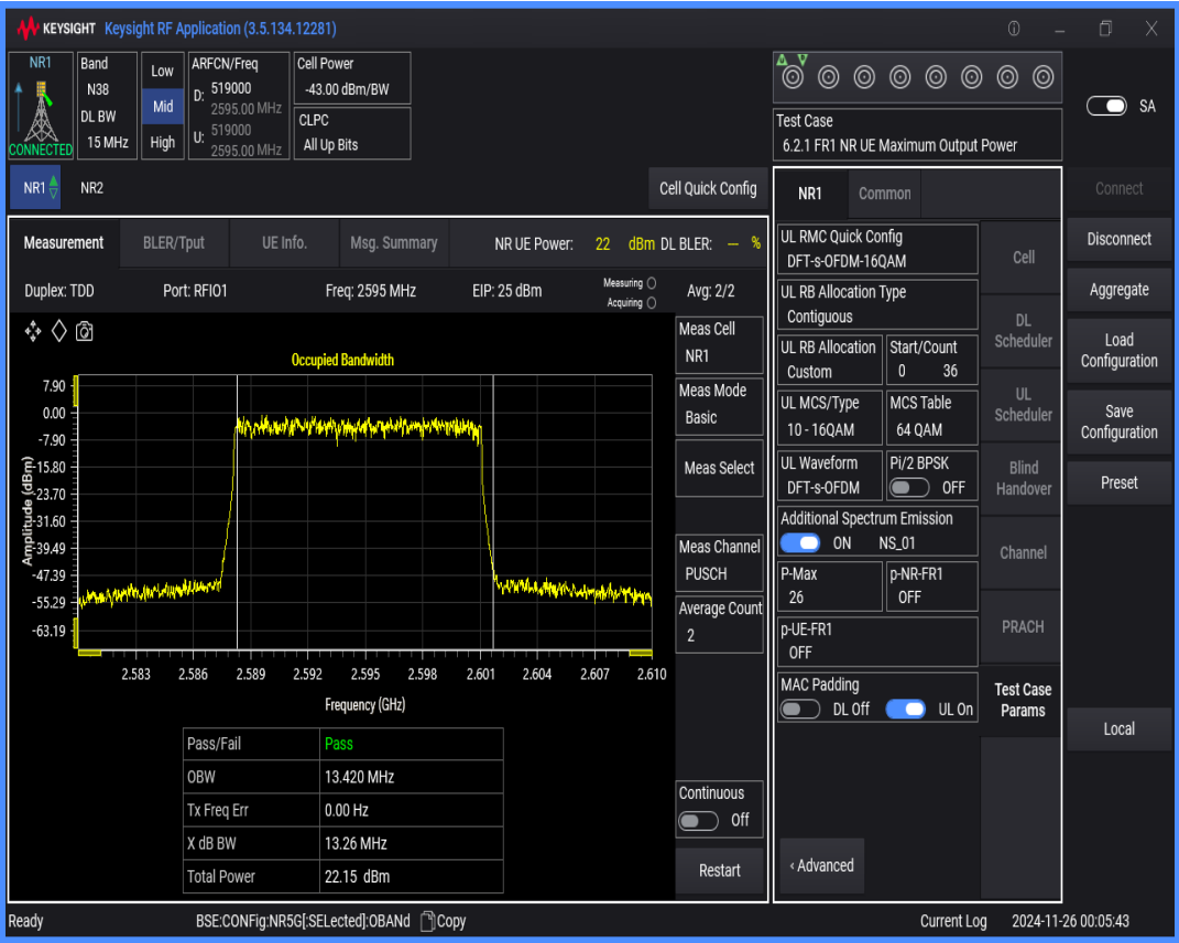
n38 SCS=30kHz DFT_QAM16 BW=10MHz Channel=519000 RB=24@0
