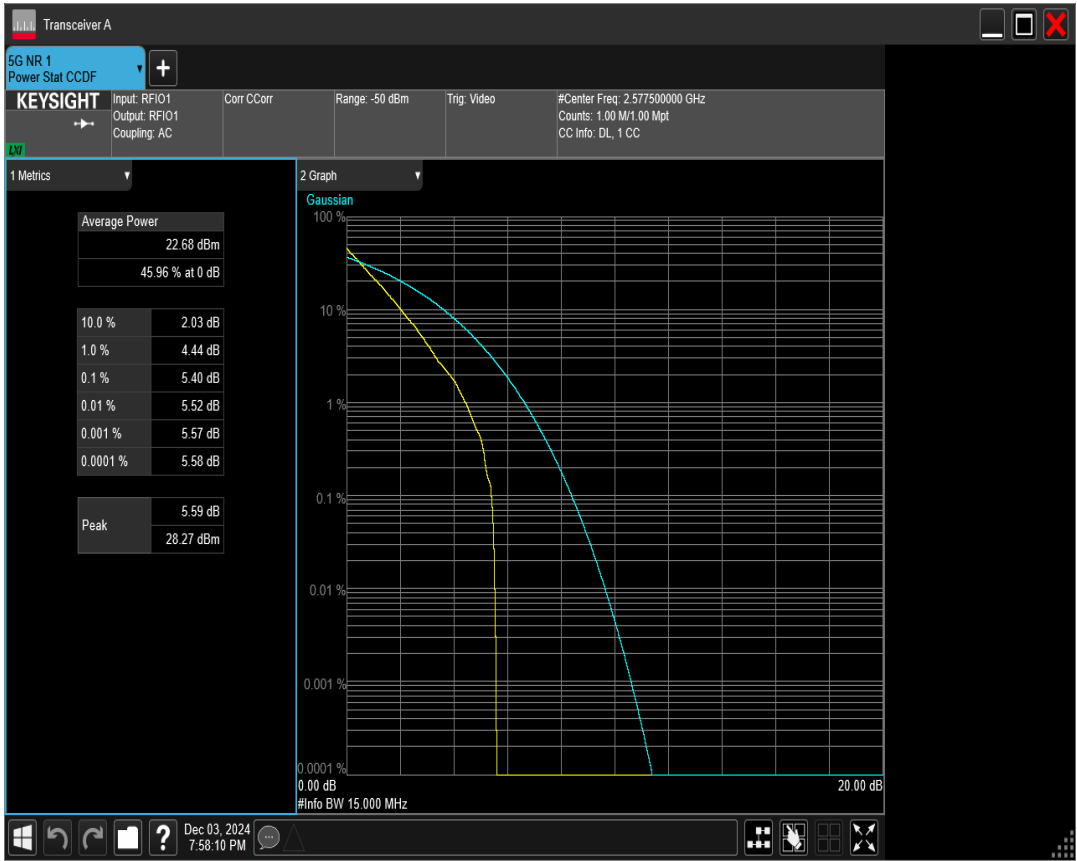
n38 SCS=30kHz DFT_BPSK BW=15MHz Channel=522500 RB=36@0
