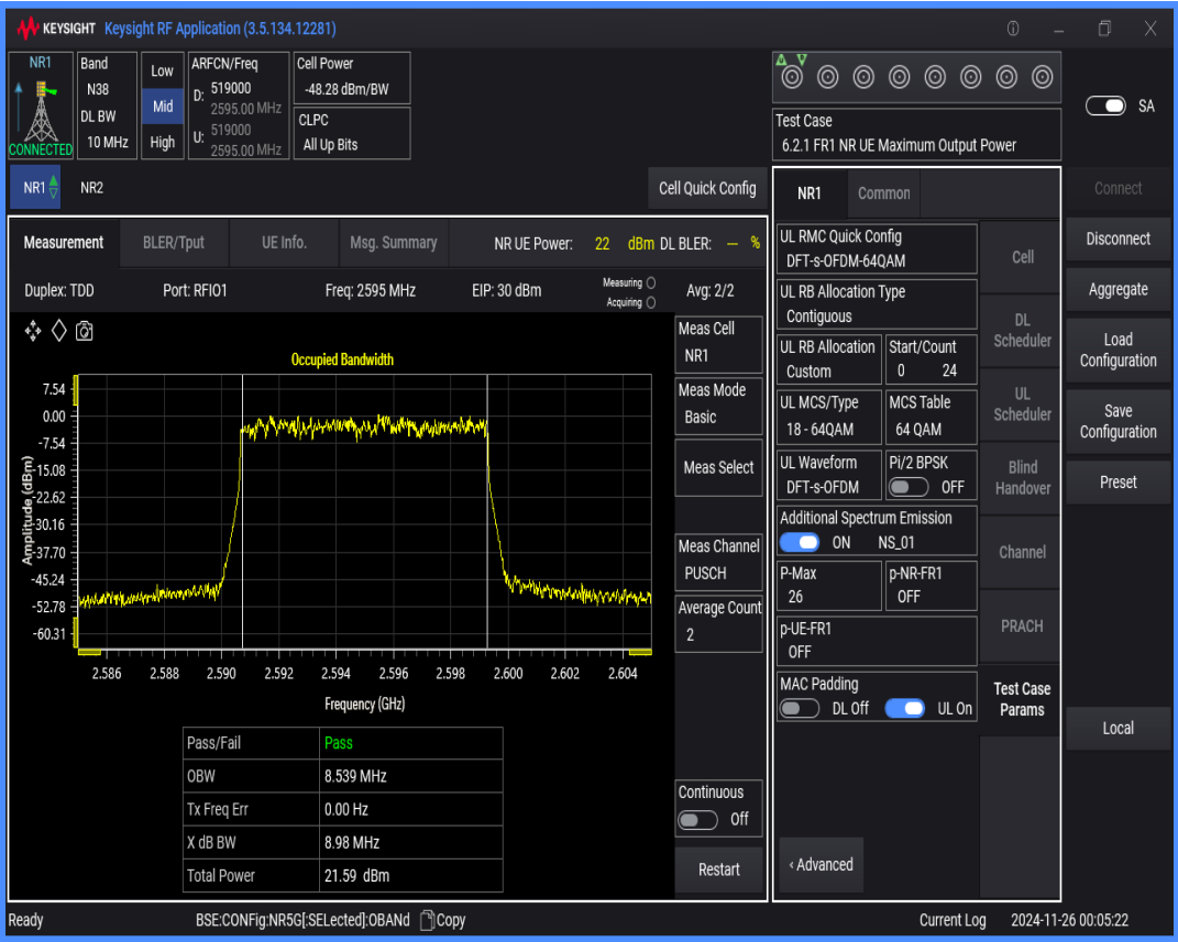
n38 SCS=30kHz DFT_QAM64 BW=15MHz Channel=519000 RB=36@0
