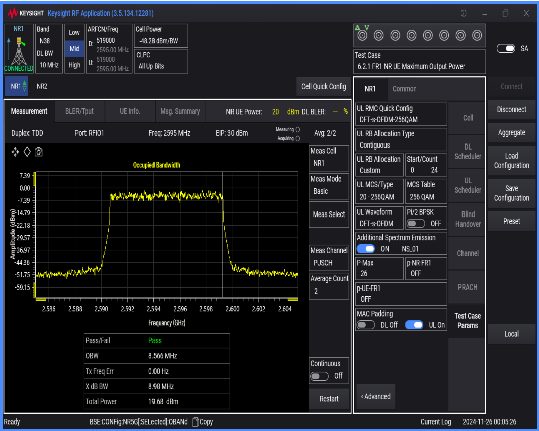
n38 SCS=30kHz DFT_QAM256 BW=15MHz Channel=519000 RB=36@0
