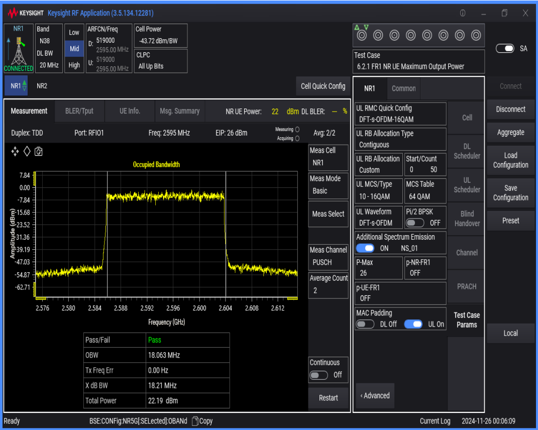
n38 SCS=30kHz DFT_QAM16 BW=15MHz Channel=519000 RB=36@0
