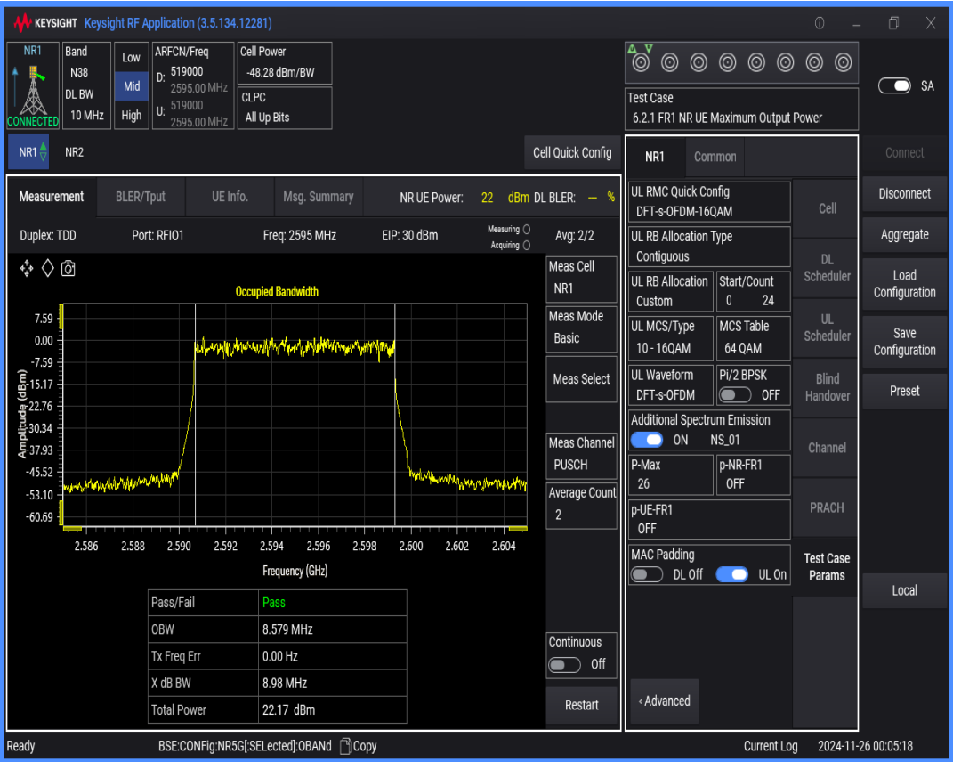
n38 SCS=30kHz DFT_QAM64 BW=10MHz Channel=519000 RB=24@0
