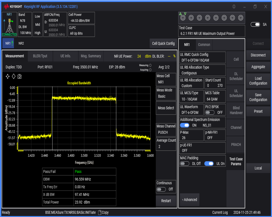
n78(3450-3550) SCS=30kHz DFT_QAM16 BW=10MHz Channel=633334 RB=24@0
