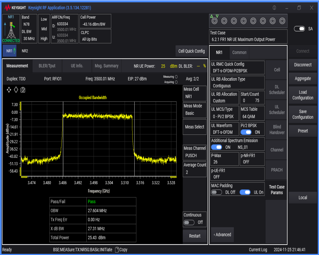
n78(3450-3550) SCS=30kHz DFT_BPSK BW=60MHz Channel=633334 RB=162@0
