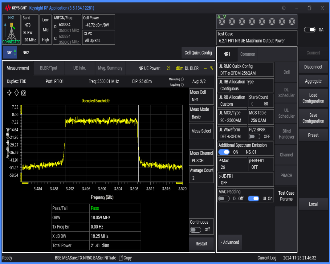
n78(3450-3550) SCS=30kHz DFT_QAM256 BW=15MHz Channel=633334 RB=36@0
