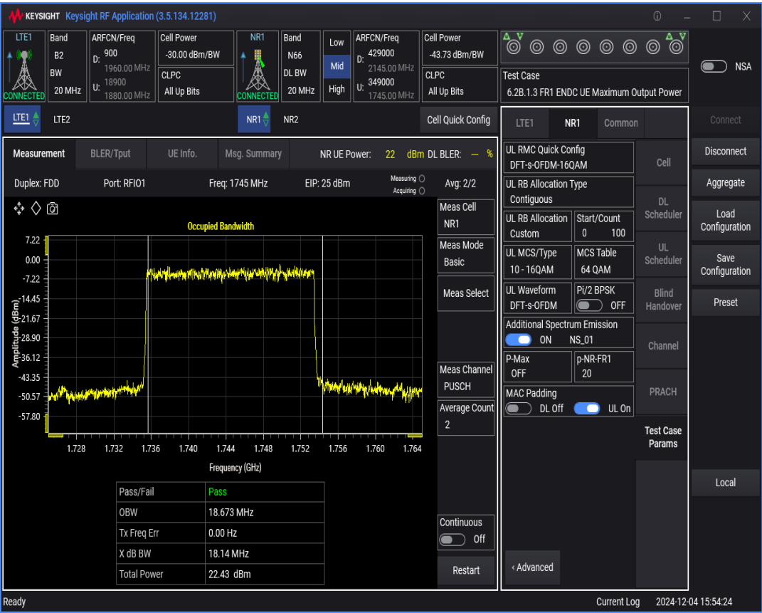
n66 SCS=15kHz DFT_QAM16 BW=15MHz Channel=349000 RB=75@0
