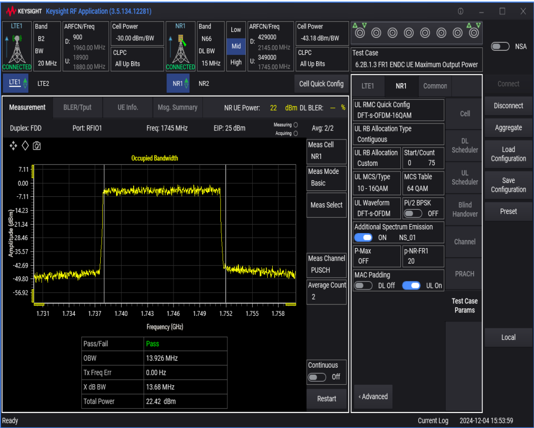
n66 SCS=15kHz DFT_QAM64 BW=20MHz Channel=349000 RB=100@0
