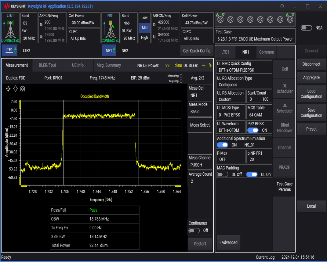
n66 SCS=15kHz DFT_BPSK BW=40MHz Channel=349000 RB=216@0
