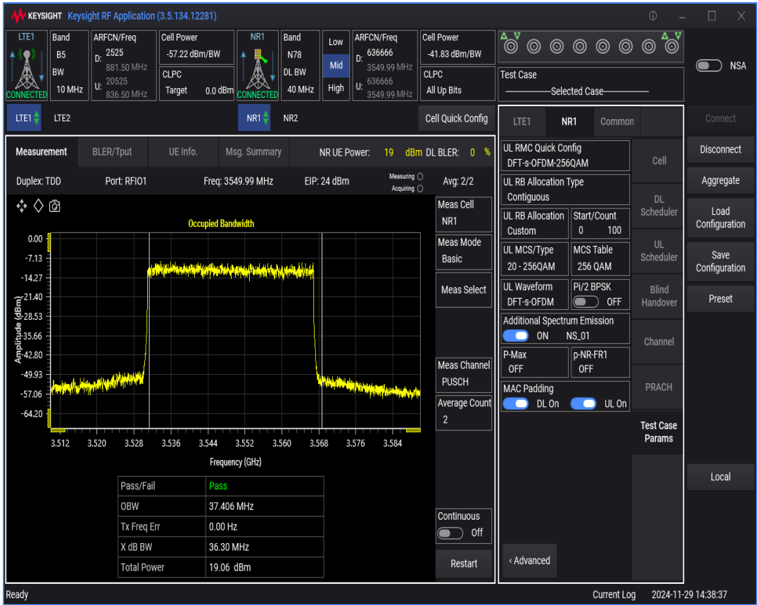
n78 SCS=30kHz DFT_QAM256 BW=50MHz Channel=636666 RB=128@0
