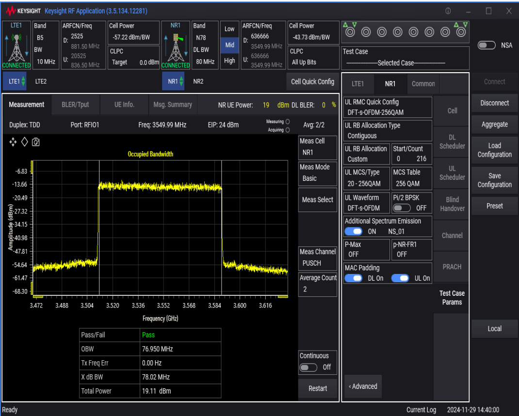
n78 SCS=30kHz DFT_QAM256 BW=60MHz Channel=636666 RB=162@0
