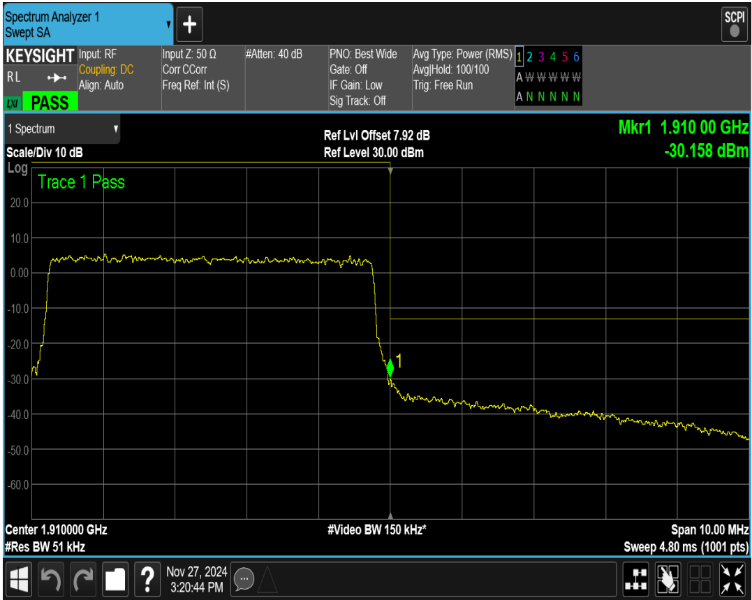
Band2 QPSK BW=5MHz Channel=19175 RB Size=25 Position=#0
