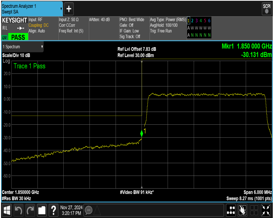
Band2 QPSK BW=5MHz Channel=19175 RB Size=25 Position=#0
