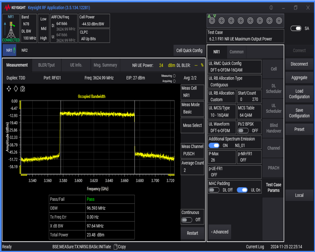
n78(3550-3700) SCS=30kHz DFT_QAM16 BW=15MHz Channel=641666 RB=36@0
