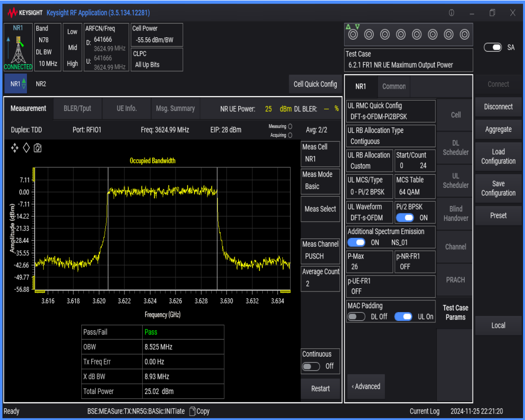
n78(3550-3700) SCS=30kHz DFT_BPSK BW=15MHz Channel=641666 RB=36@0
