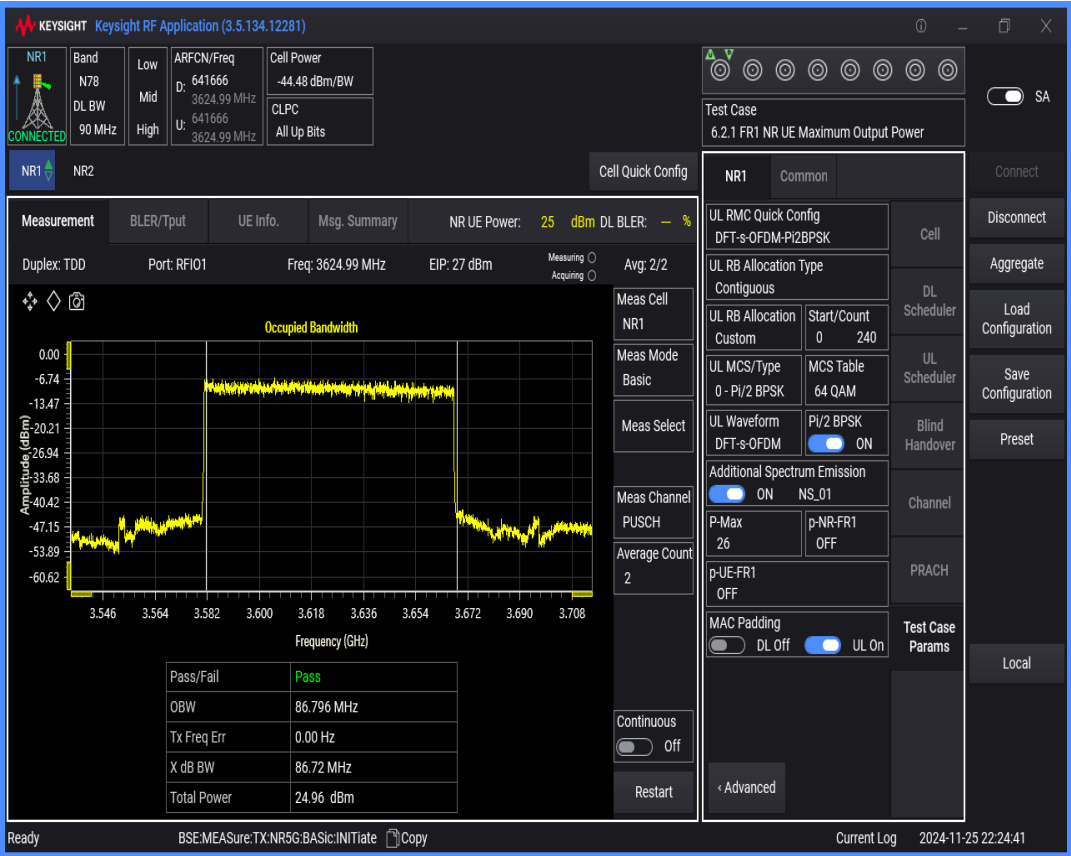
n78(3550-3700) SCS=30kHz DFT_QAM16 BW=10MHz Channel=641666 RB=24@0
