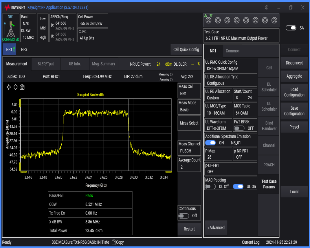
n78(3550-3700) SCS=30kHz DFT_QAM16 BW=100MHz Channel=641666 RB=270@0
