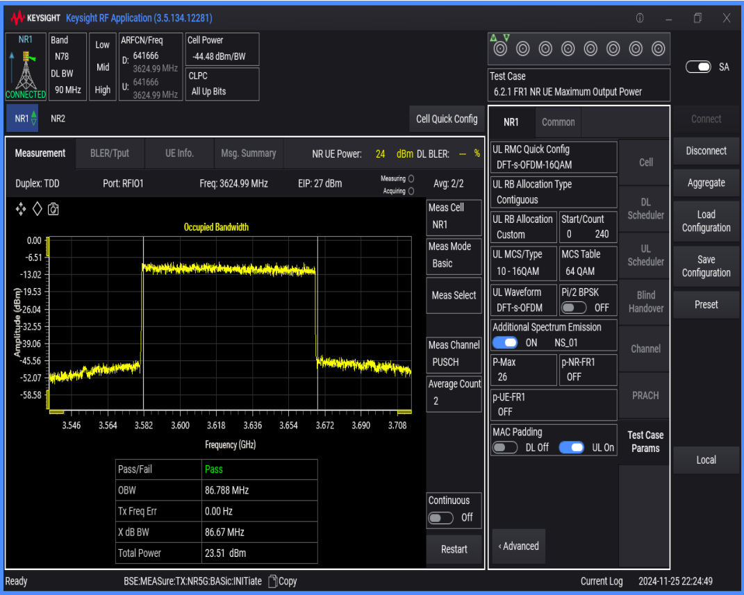
n78(3550-3700) SCS=30kHz DFT_QAM16 BW=80MHz Channel=641666 RB=216@0
