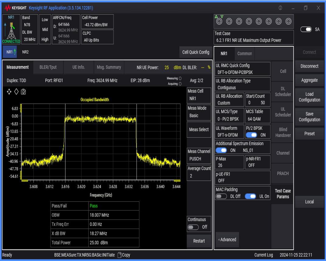
n78(3550-3700) SCS=30kHz DFT_BPSK BW=50MHz Channel=641666 RB=128@0
