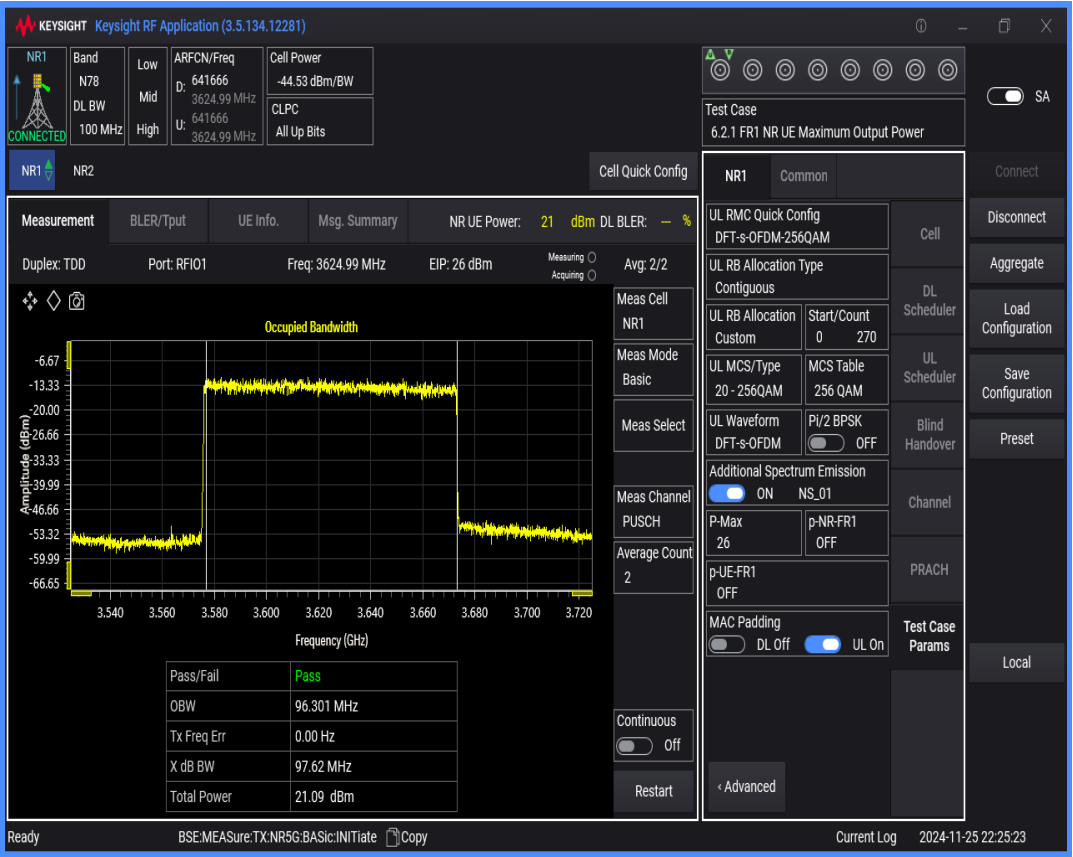
n78(3550-3700) SCS=30kHz DFT_QAM256 BW=40MHz Channel=641666 RB=100@0
