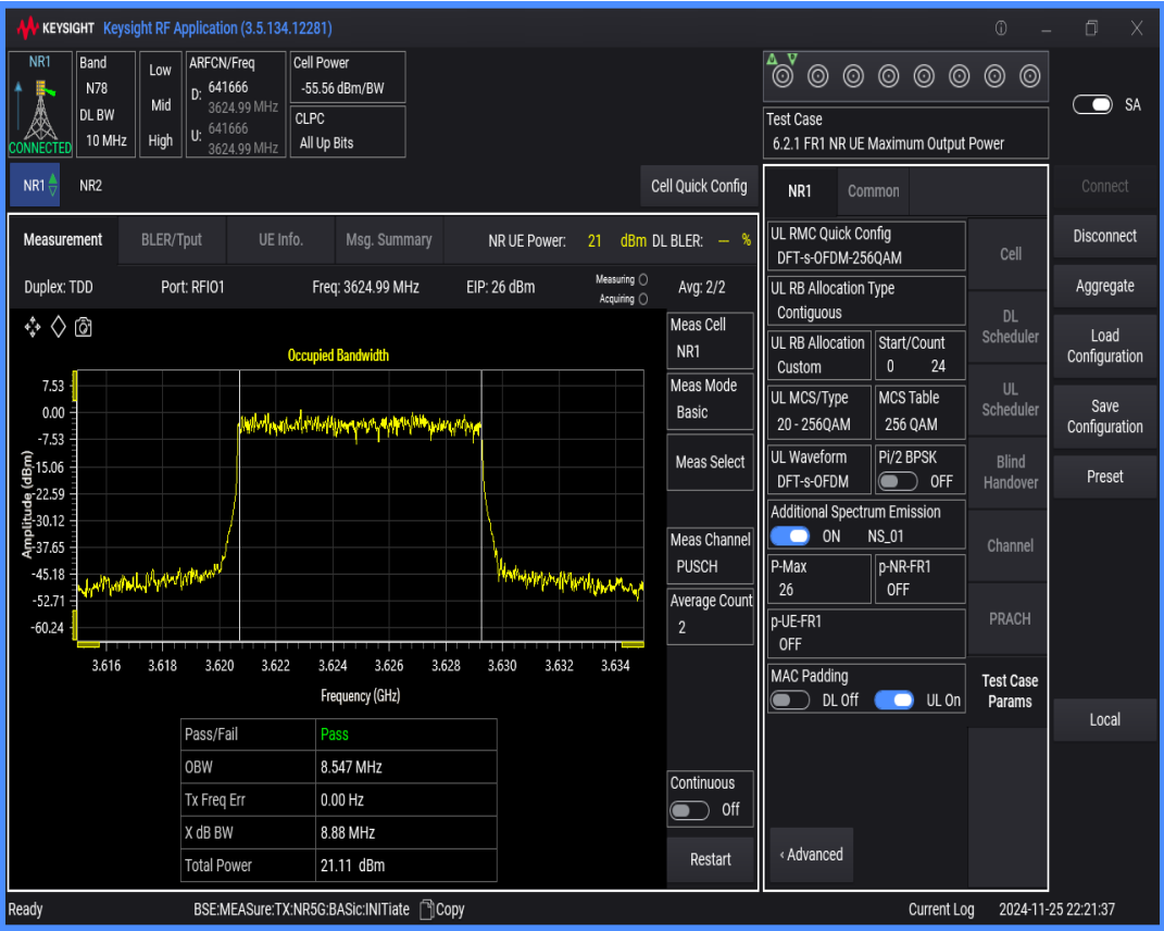
n78(3550-3700) SCS=30kHz DFT_QAM256 BW=15MHz Channel=641666 RB=36@0
