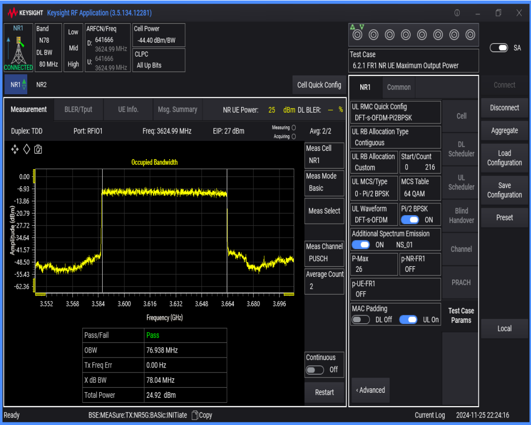
n78(3550-3700) SCS=30kHz DFT_BPSK BW=90MHz Channel=641666 RB=240@0
