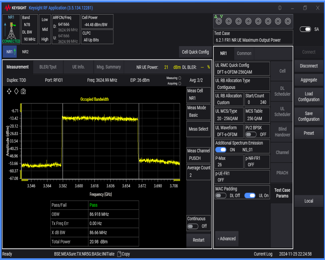
n78(3550-3700) SCS=30kHz DFT_QAM64 BW=100MHz Channel=641666 RB=270@0
