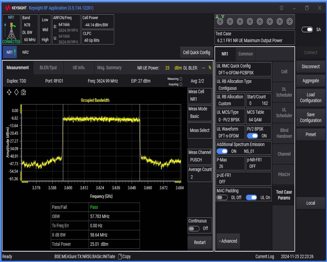
n78(3550-3700) SCS=30kHz DFT_BPSK BW=80MHz Channel=641666 RB=216@0
