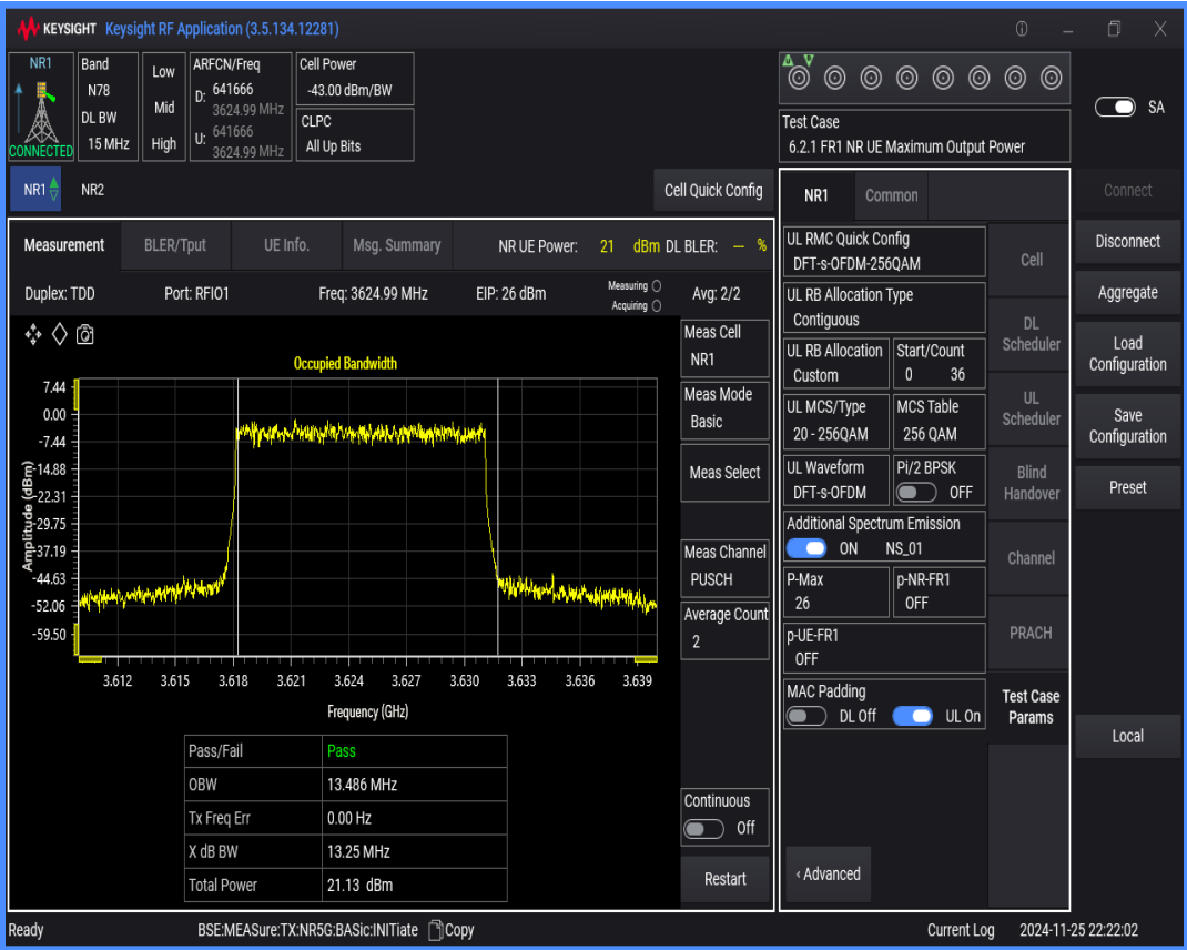
n78(3550-3700) SCS=30kHz DFT_QAM256 BW=90MHz Channel=641666 RB=240@0
