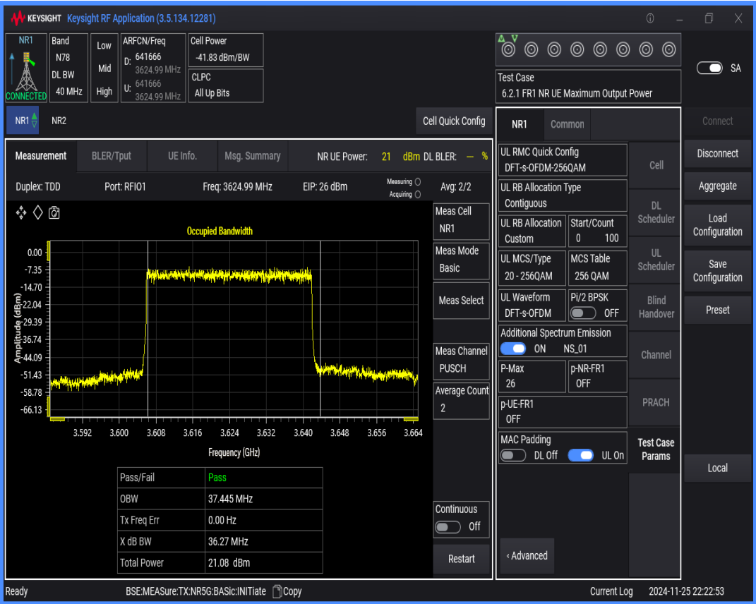
n78(3550-3700) SCS=30kHz DFT_QAM256 BW=50MHz Channel=641666 RB=128@0
