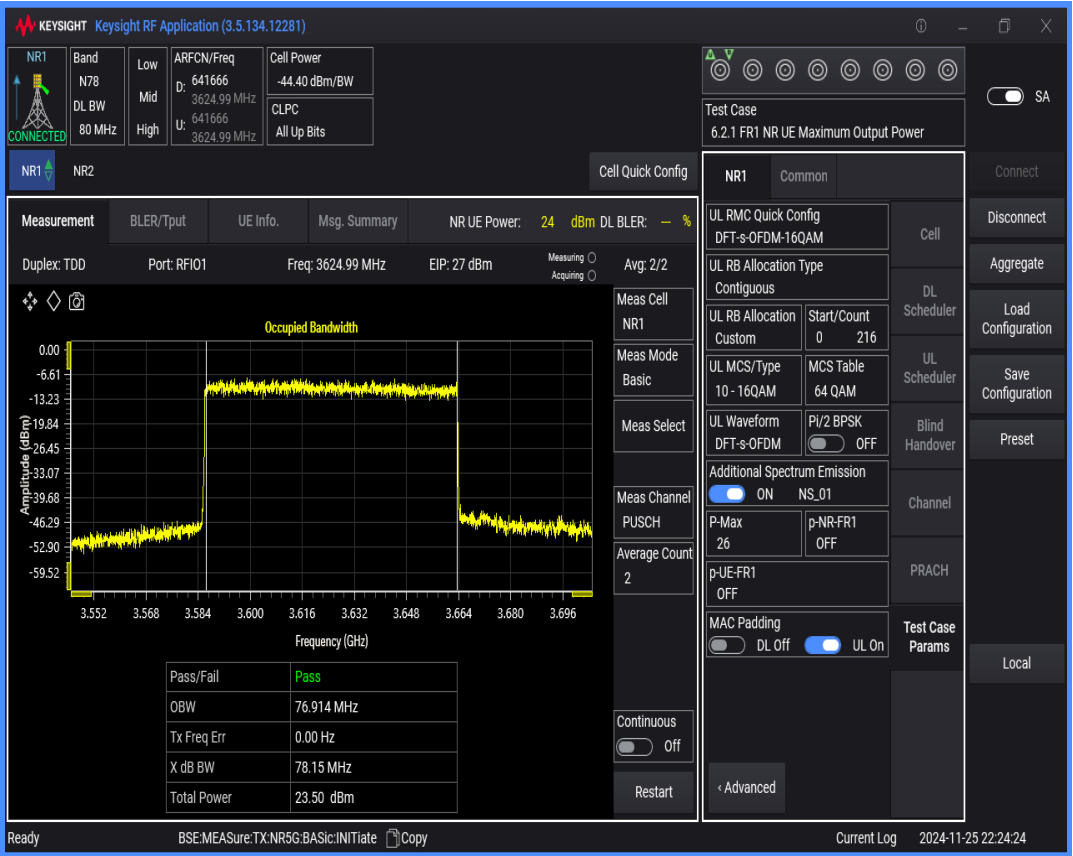
n78(3550-3700) SCS=30kHz DFT_QAM256 BW=100MHz Channel=641666 RB=270@0
