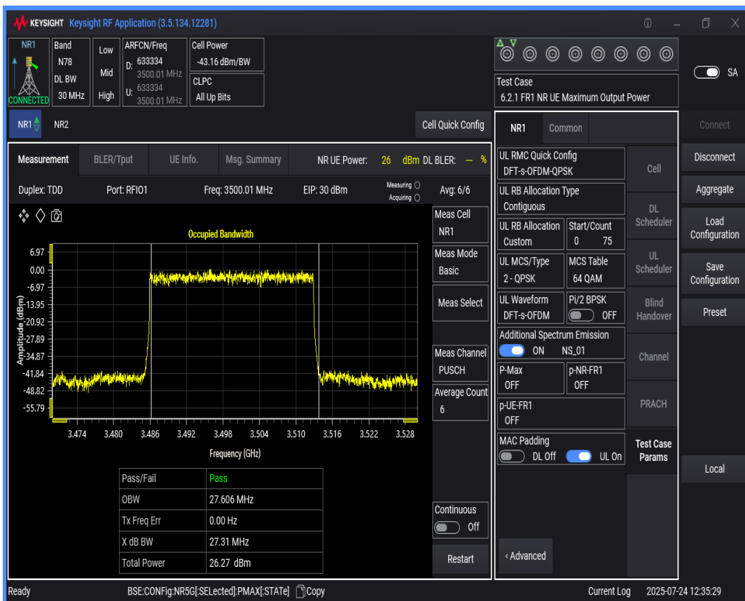
n78(3450-3550) SCS=30kHz DFT_QPSK BW=15MHz Channel=633334 RB=36 @0
