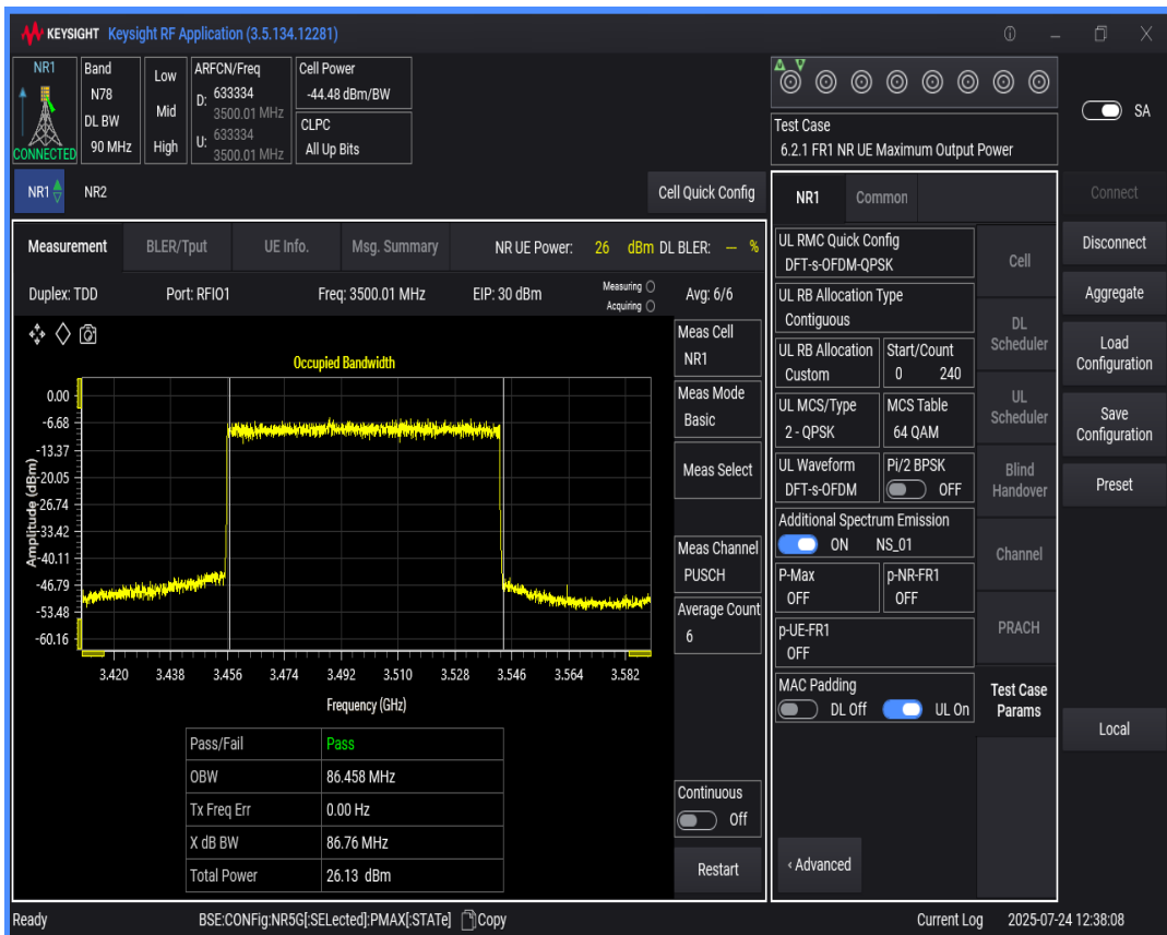
n78(3450-3550) SCS=30kHz DFT_QPSK BW=60MHz Channel=633334 RB=162@0
