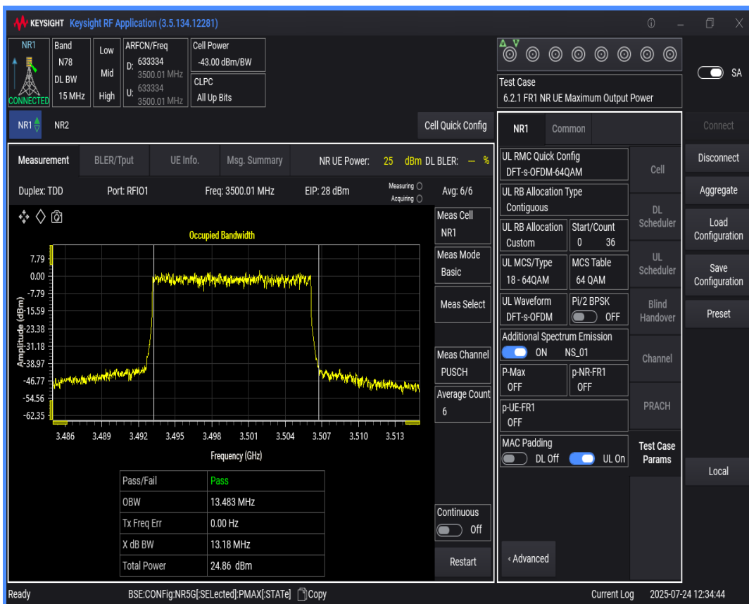
n78(3450-3550) SCS=30kHz DFT_QAM64 BW=20MHz Channel=633334 RB=50@0
