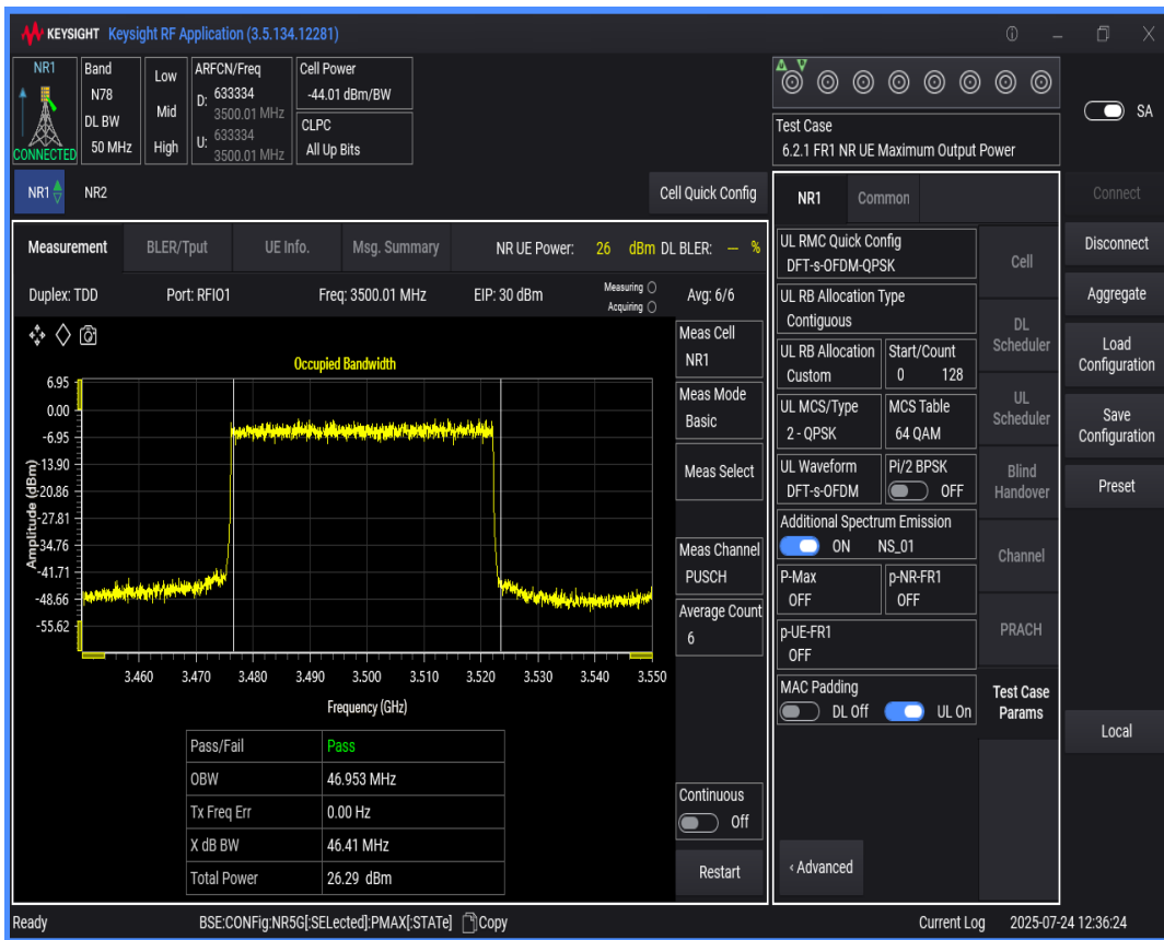
n78(3450-3550) SCS=30kHz DFT_QPSK BW=30MHz Channel=633334 RB=75 @0
