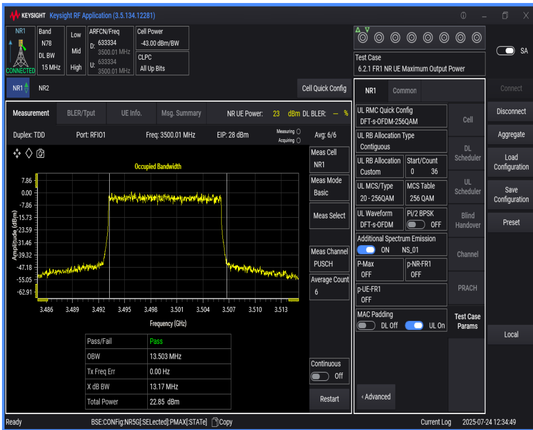
n78(3450-3550) SCS=30kHz DFT_QAM256 BW=10MHz Channel=633334 RB=24@0
