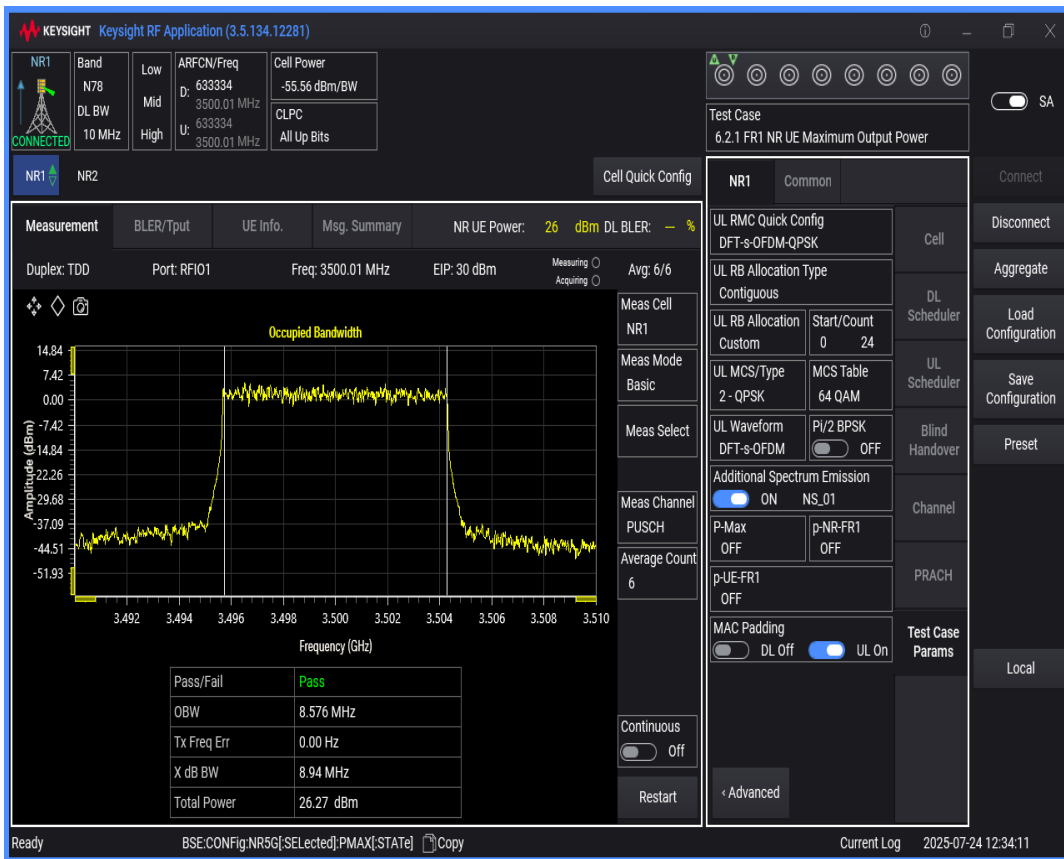
n78(3450-3550) SCS=30kHz DFT_QAM64 BW=80MHz Channel=633334 RB=216@0
