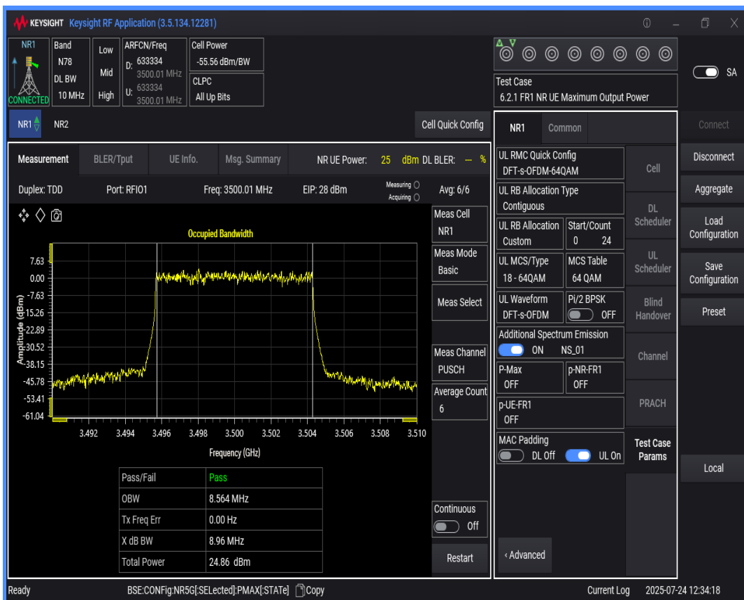
n78(3450-3550) SCS=30kHz DFT_QAM256 BW=90MHz Channel=633334 RB=240@0
