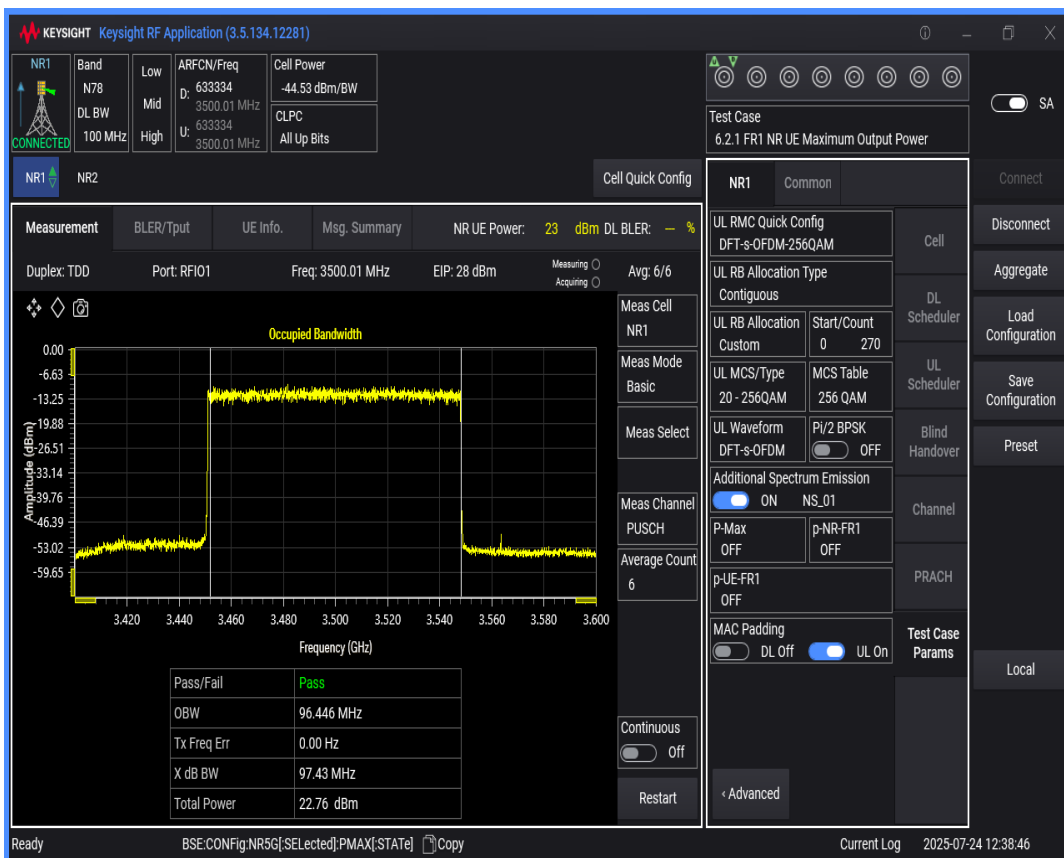
n78(3450-3550) SCS=30kHz DFT_QAM16 BW=70MHz Channel=633334 RB=180@0
