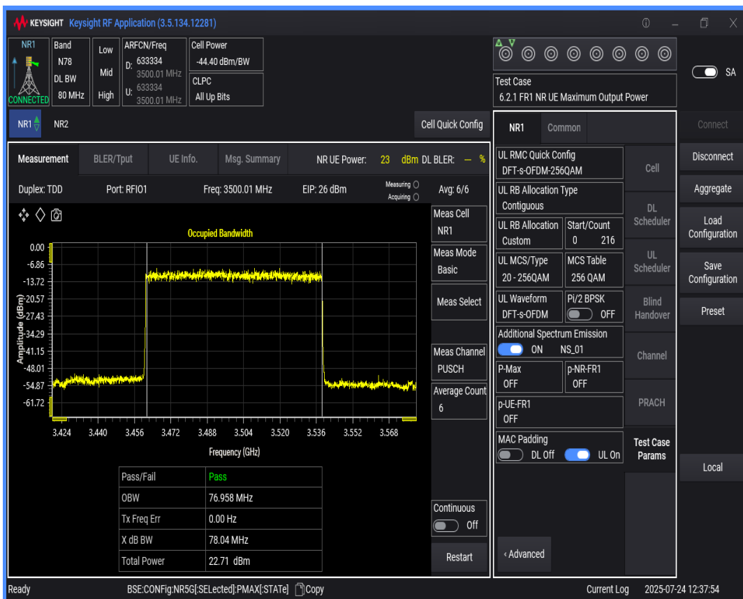
n78(3450-3550) SCS=30kHz DFT_QAM256 BW=60MHz Channel=633334 RB=162 @0
