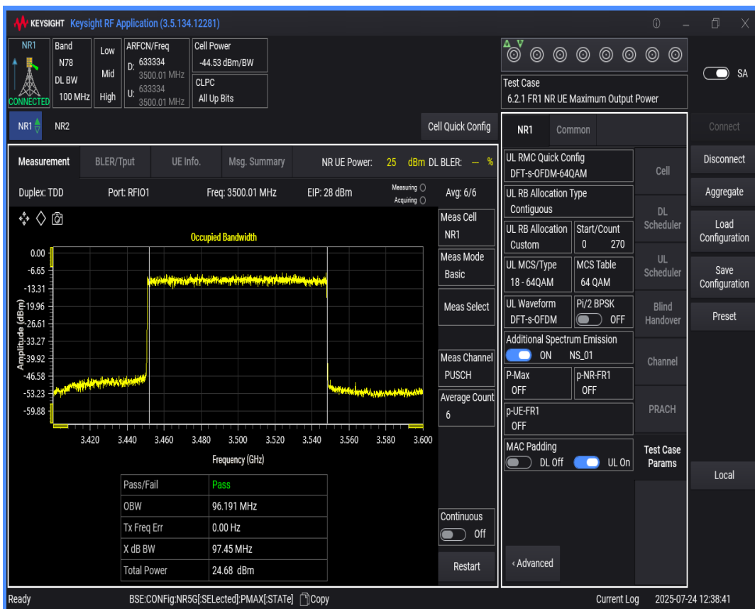
n78(3450-3550) SCS=30kHz DFT_QAM64 BW=50MHz Channel=633334 RB=128 @0
