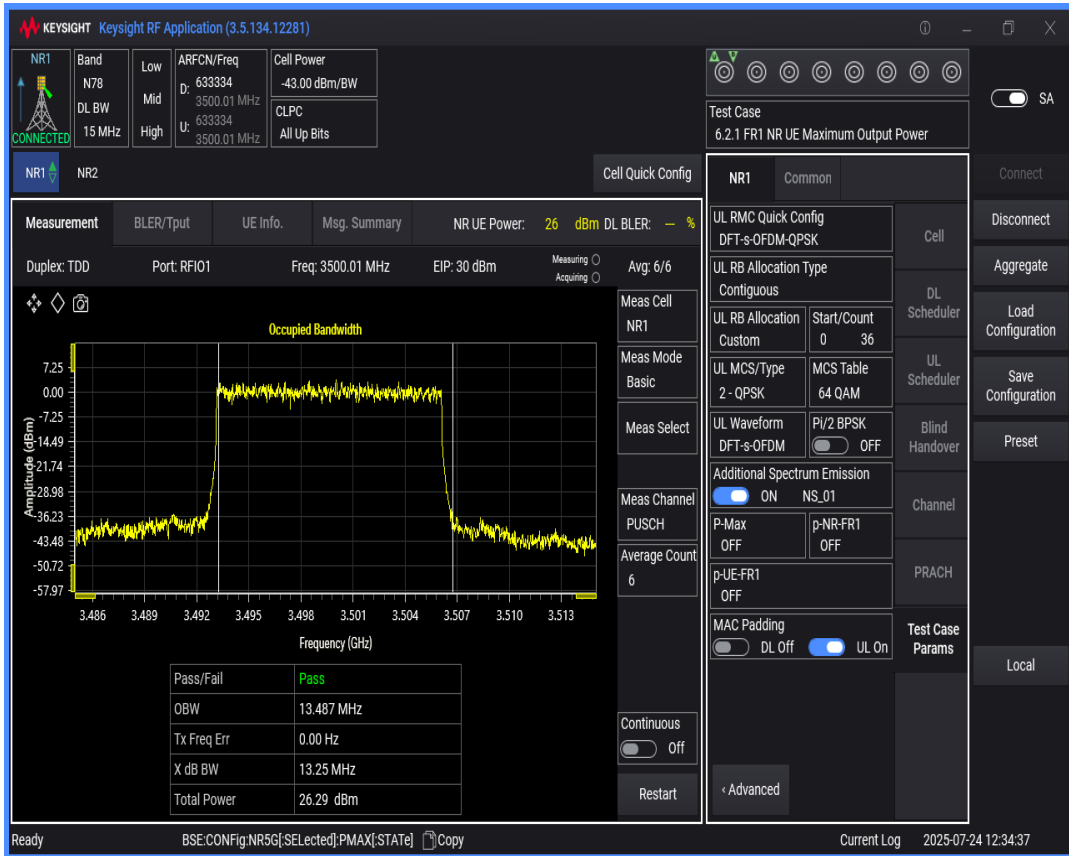
n78(3450-3550) SCS=30kHz DFT_QPSK BW=20MHz Channel=633334 RB=50 @0
