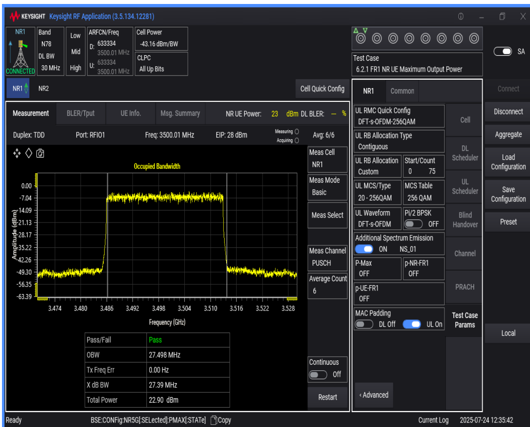
n78(3450-3550) SCS=30kHz DFT_QAM256 BW=70MHz Channel=633334 RB=180@0
