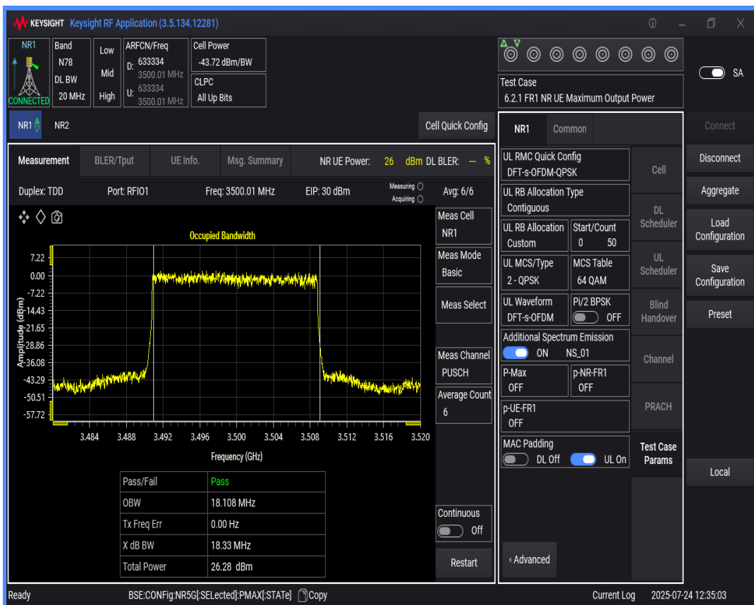
n78(3450-3550) SCS=30kHz DFT_QPSK BW=80MHz Channel=633334 RB=216 @0
