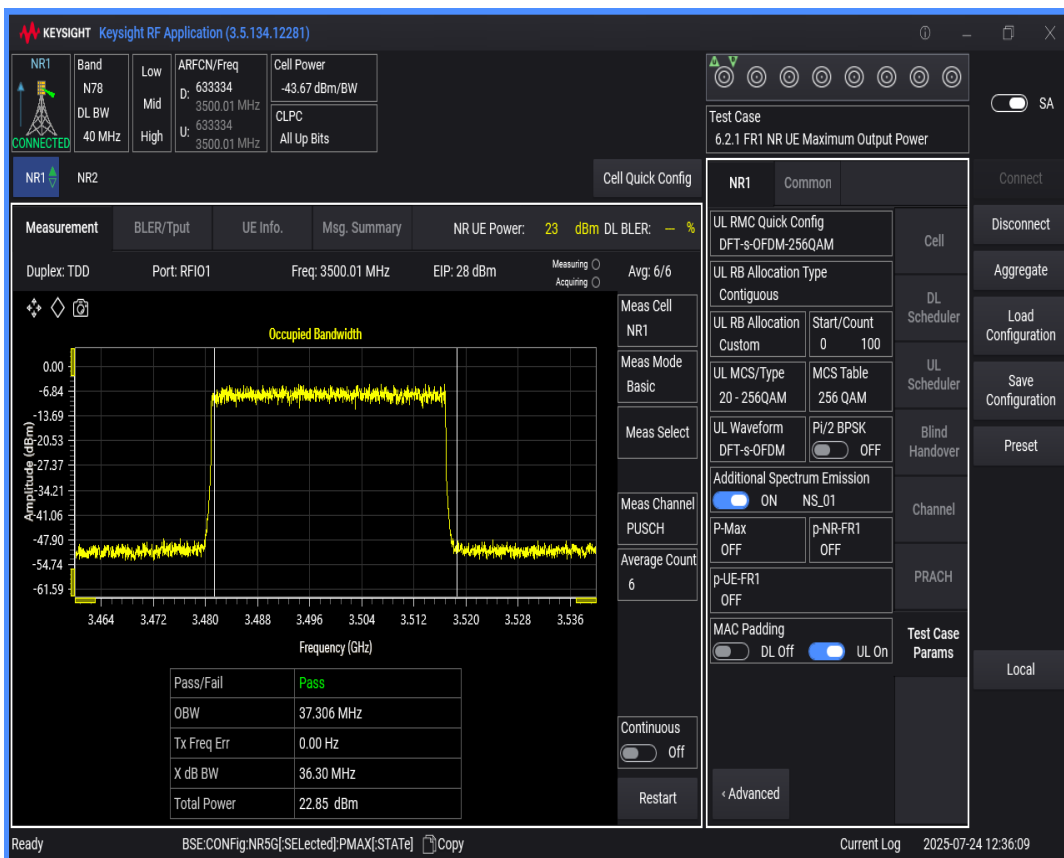
n78(3450-3550) SCS=30kHz DFT_QAM256 BW=50MHz Channel=633334 RB=128@0
