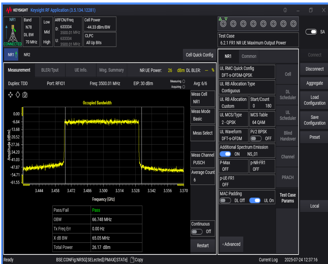
n78(3450-3550) SCS=30kHz DFT_QPSK BW=70MHz Channel=633334 RB=180@0
