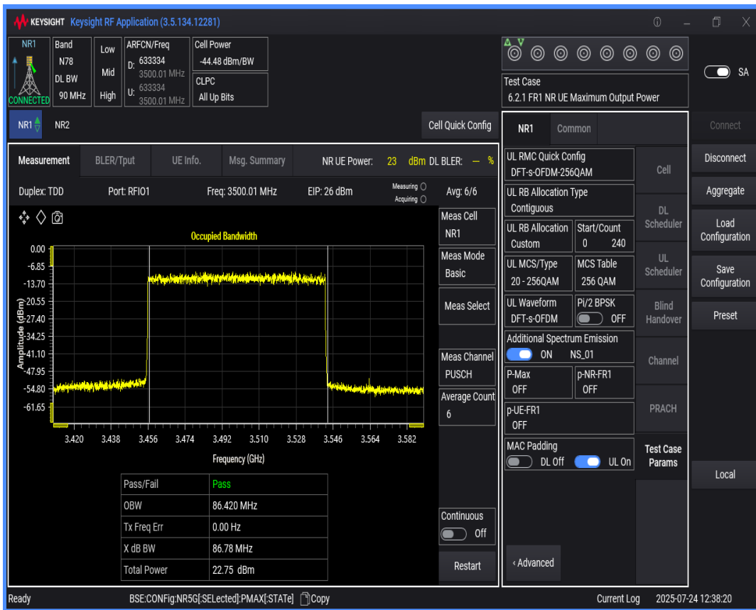
n78(3450-3550) SCS=30kHz DFT_QAM64 BW=100MHz Channel=633334 RB=270 @0
