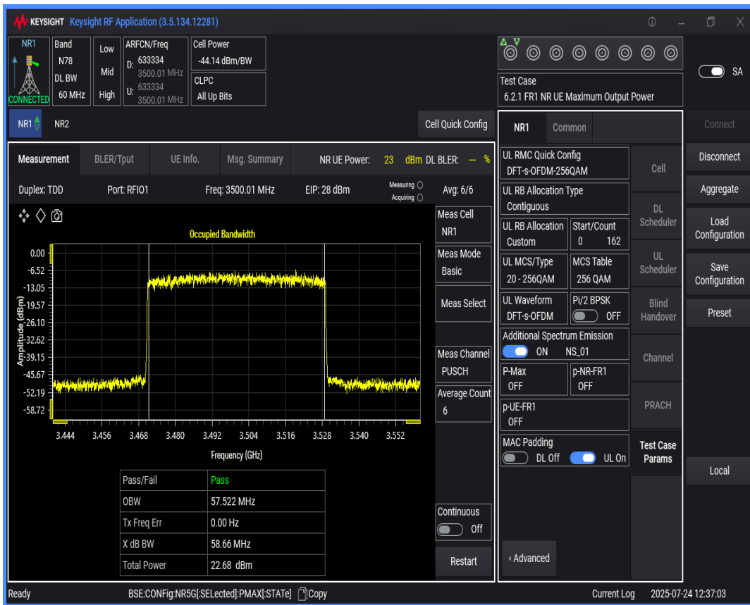
n78(3450-3550) SCS=30kHz DFT_QAM256 BW=40MHz Channel=633334 RB=100@0
