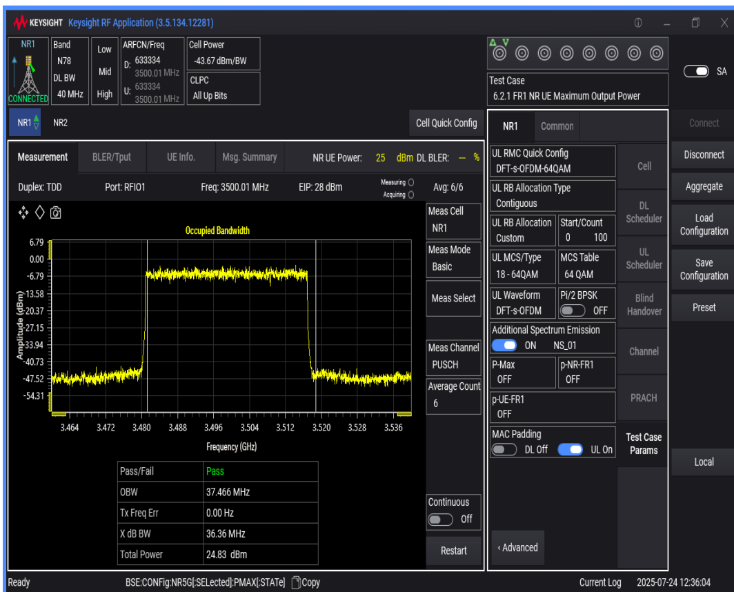
n78(3450-3550) SCS=30kHz DFT_QAM64 BW=70MHz Channel=633334 RB=180@0
