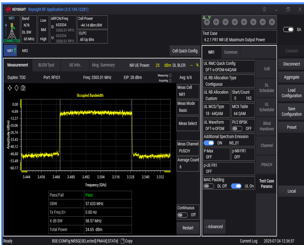
n78(3450-3550) SCS=30kHz DFT_QAM64 BW=30MHz Channel=633334 RB=75 @0
