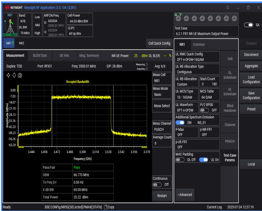
n78(3450-3550) SCS=30kHz DFT_QAM16 BW=80MHz Channel=633334 RB=216@0
