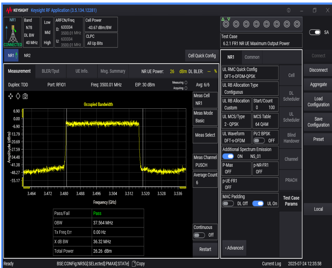
n78(3450-3550) SCS=30kHz DFT_QPSK BW=50MHz Channel=633334 RB=128@0
