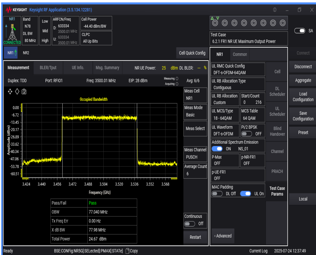
n78(3450-3550) SCS=30kHz DFT_QAM64 BW=90MHz Channel=633334 RB=240@0
