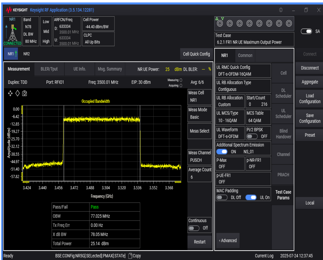
n78(3450-3550) SCS=30kHz DFT_QAM256 BW=15MHz Channel=633334 RB=36@0
