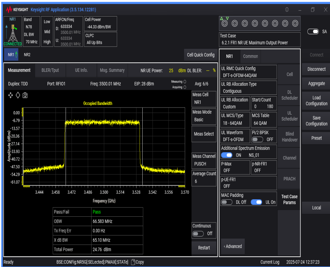
n78(3450-3550) SCS=30kHz DFT_QPSK BW=100MHz Channel=633334 RB=270@0
