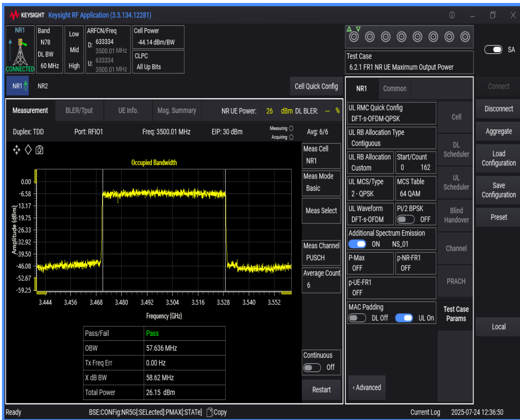
n78(3450-3550) SCS=30kHz DFT_QPSK BW=70MHz Channel=633334 RB=180@0
