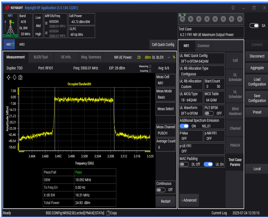
n78(3450-3550) SCS=30kHz DFT_QAM64 BW=10MHz Channel=633334 RB=24@0
