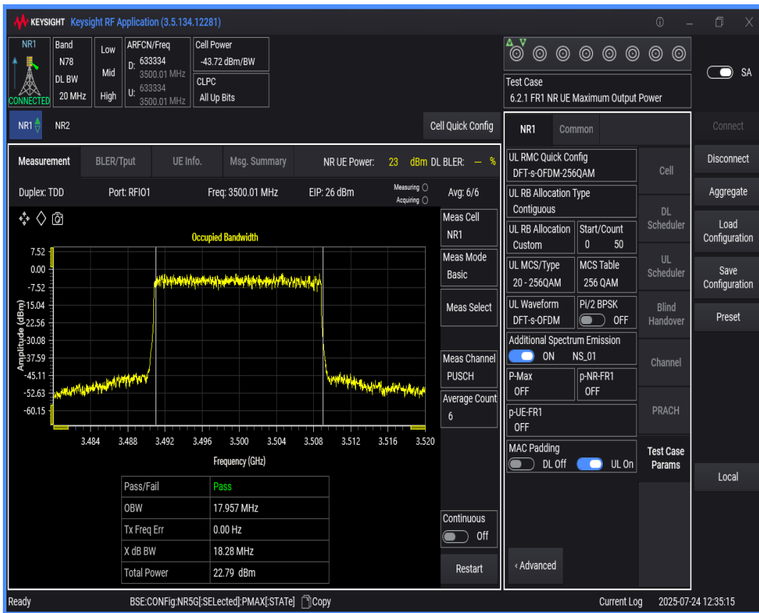
n78(3450-3550) SCS=30kHz DFT_QAM256 BW=30MHz Channel=633334 RB=75@0
