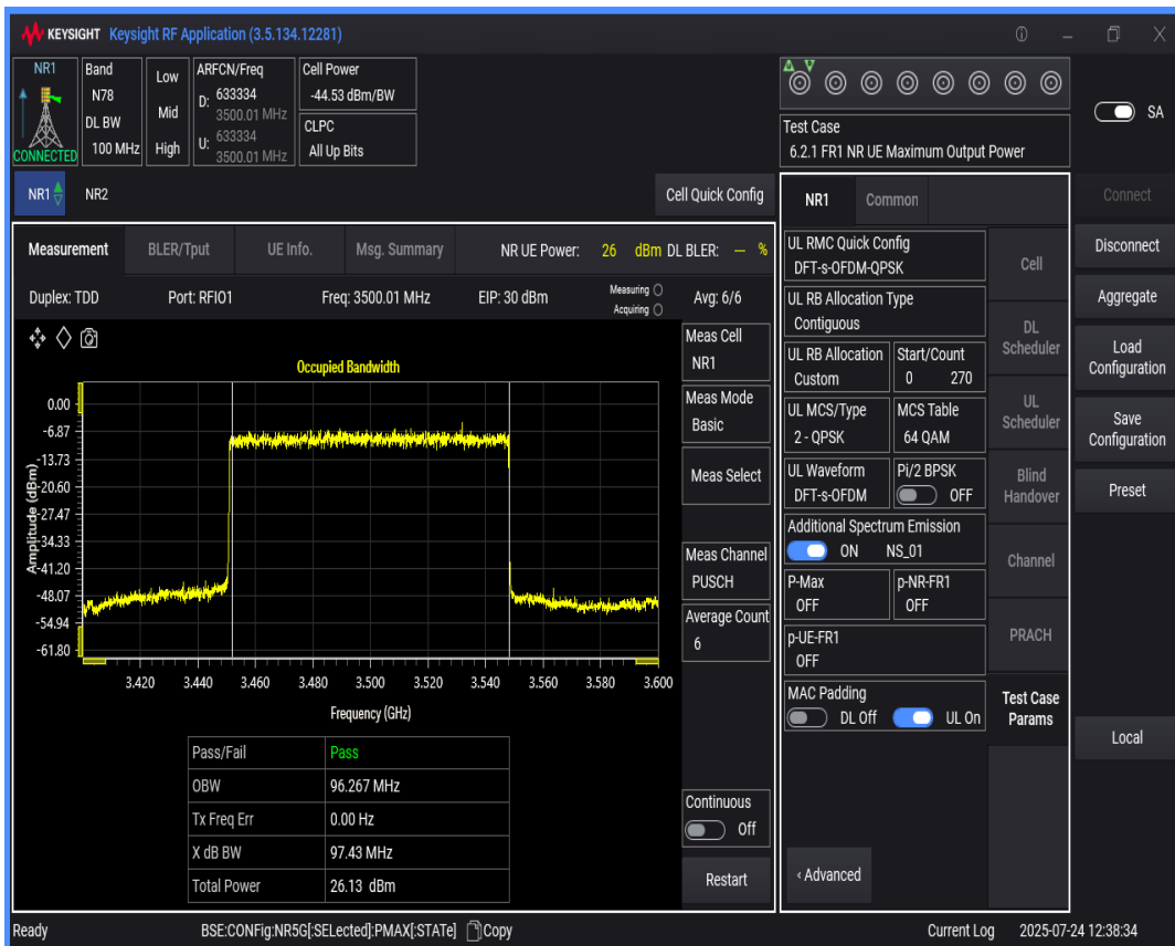
n78(3450-3550) SCS=30kHz DFT_QPSK BW=10MHz Channel=633334 RB=24@0
