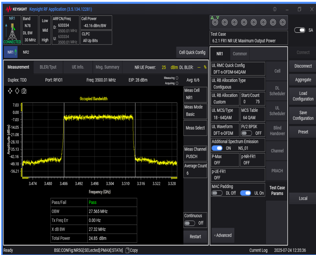
n78(3450-3550) SCS=30kHz DFT_QAM64 BW=40MHz Channel=633334 RB=100@0
