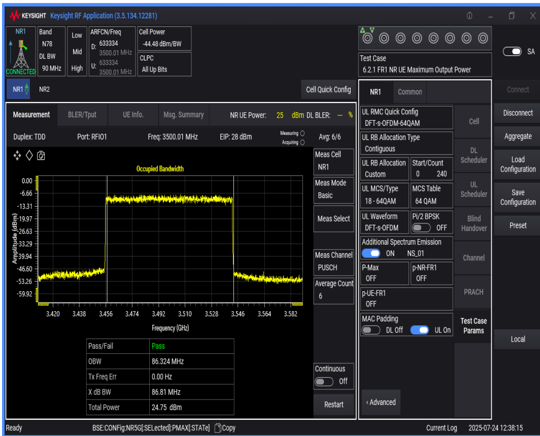
n78(3450-3550) SCS=30kHz DFT_QPSK BW=40MHz Channel=633334 RB=100@0
