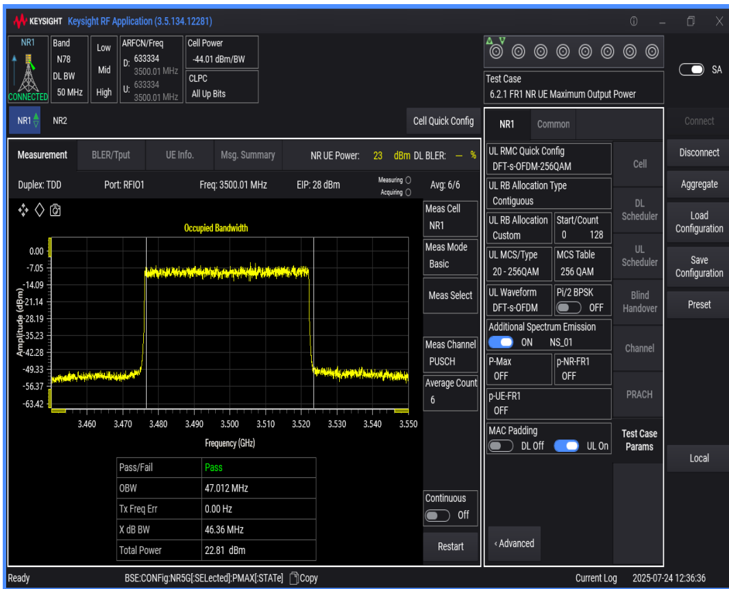
n78(3450-3550) SCS=30kHz DFT_QAM64 BW=15MHz Channel=633334 RB=36@0
