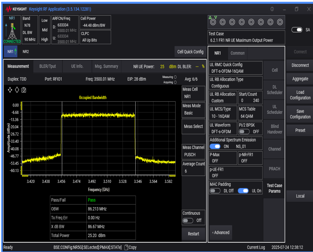
n78(3450-3550) SCS=30kHz DFT_QAM256 BW=100MHz Channel=633334 RB=270@0
