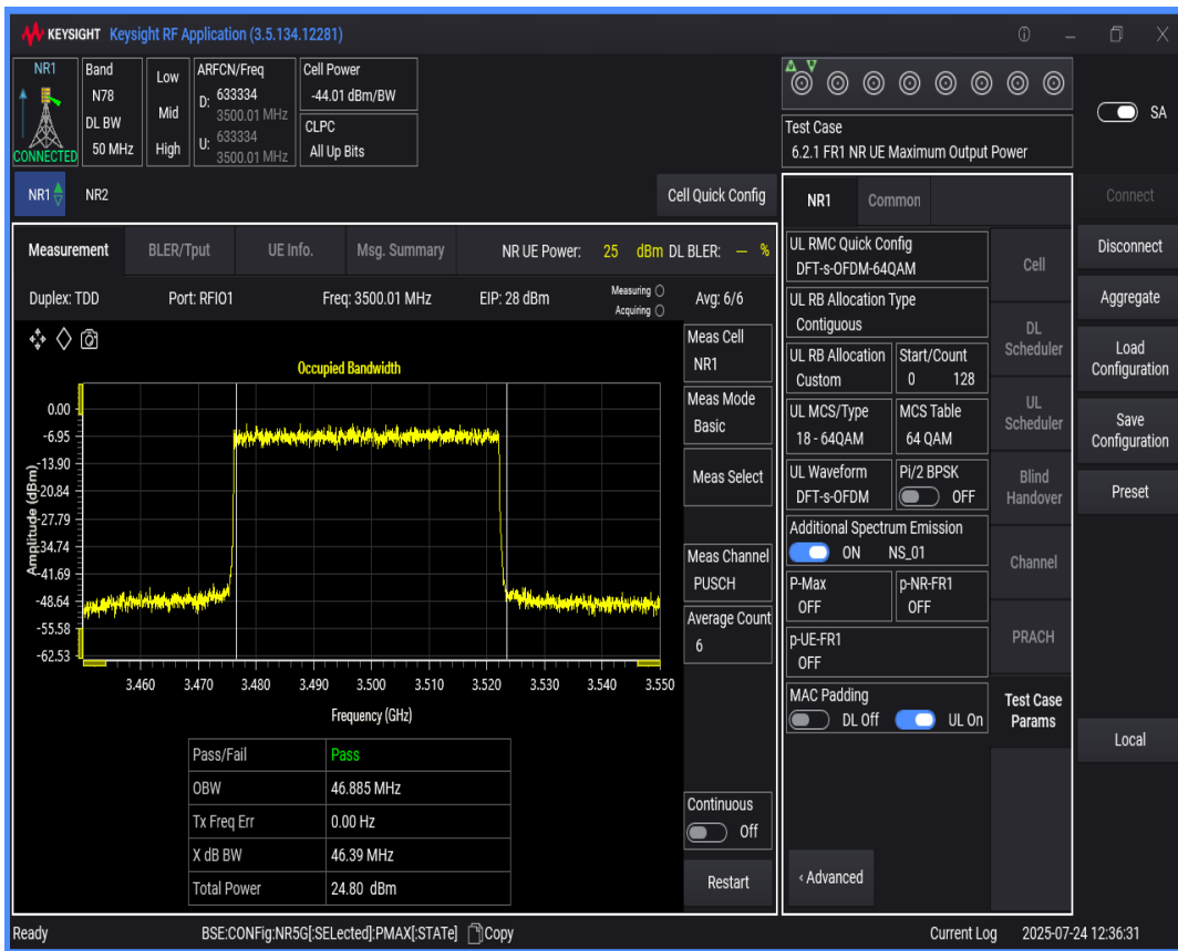
n78(3450-3550) SCS=30kHz DFT_QAM64 BW=60MHz Channel=633334 RB=162 @0
