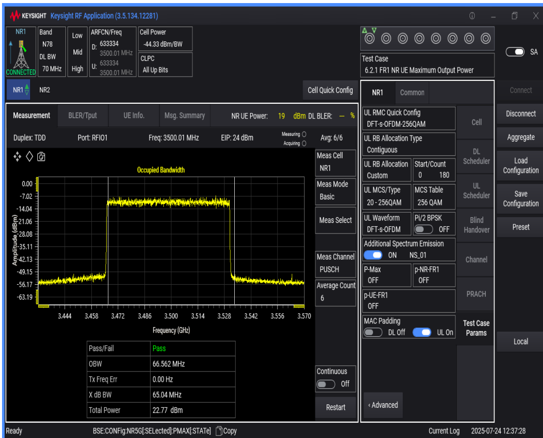
n78(3450-3550) SCS=30kHz DFT_QAM256 BW=80MHz Channel=633334 RB=216 @0
