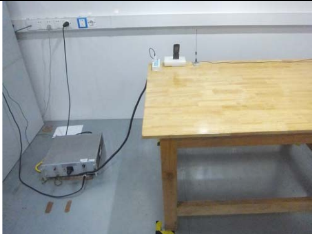
Conducted Emissions Test Setup Front View
