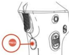
h. After pressing the trigger key, the green light will flash, and the Bluetooth icon will indicate the battery status of the gimbal.
