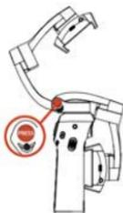
b. Twist the tilt motor and roll motor to unlock it;
