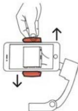
c. Make sure the camera of your phone is on the left side in case it gets stuck by the motor arm;
