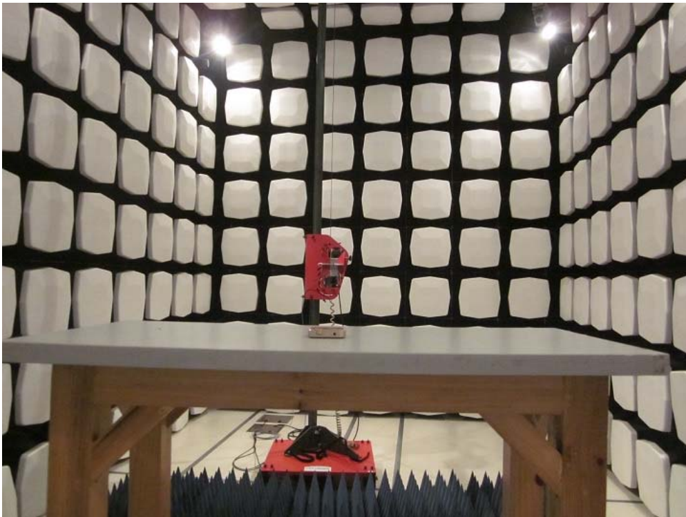
Measurement of Radiated Emission Test Set Up
