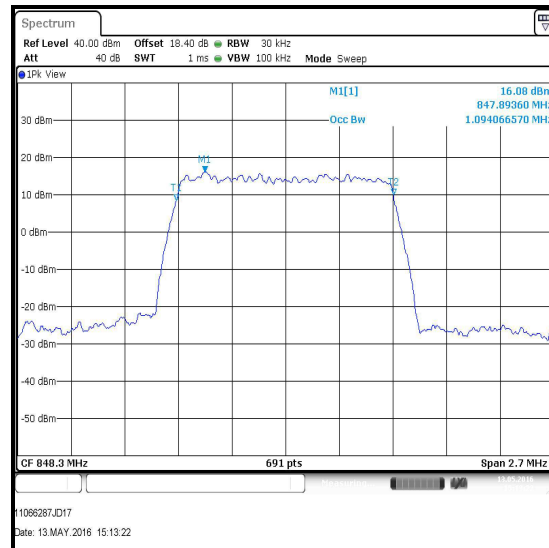
Top Channel / 16QAM
