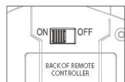
2 As shown on the picture, move the switch on the back of the remote controller to ON. After the sound of "bi", the car starting sound appeared, means the connection is successful. You can start playing with the RC car according to the instructions.
