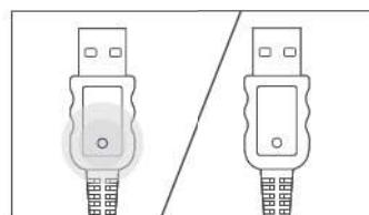
When the LED light on the USB plug keeps lighting up, the car is charging. When the light goes out, the charging is complete.
