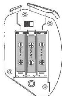
Press the lock button with a screwdriver and remove the battery cover. Loading 3\*AAA batteries according to the positive and negative directions in the picture.
