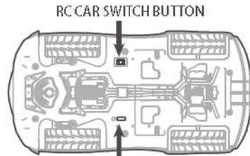
Move the car switch to the OFF side. Plug the USB cable into the computer, and plug the other part into the charging port on the car for charging.
