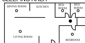
Figure 1: LOCATIONS FOR PLACING SMOKE ALARMS FOR SINGLE RESIDENCE WITH ONLY ONE SLEEPING AREA
