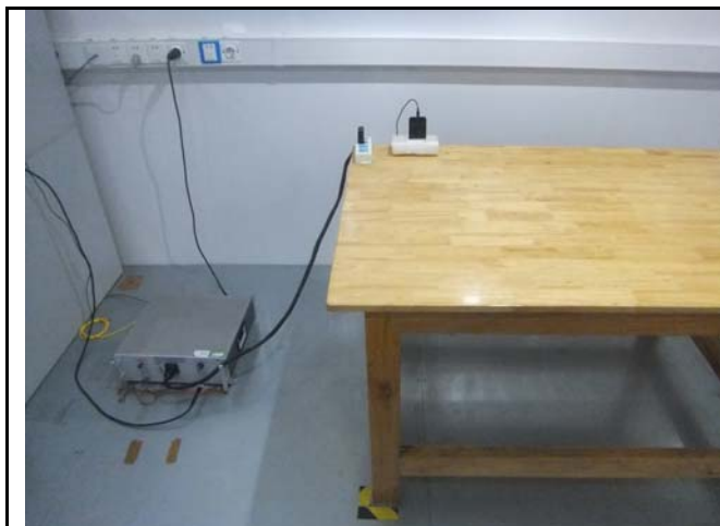
Conducted Emissions Test Setup Front View
