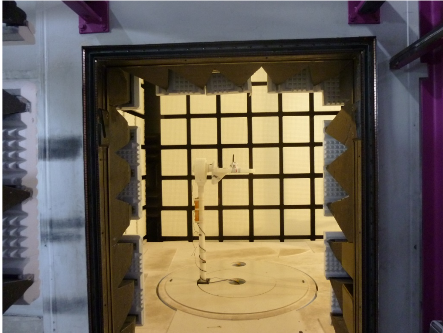
Photo 13: EUT at the anechoic chamber, metal housing (ex version)
