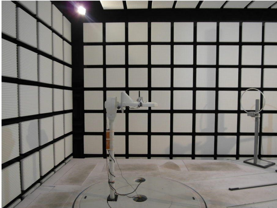
Photo 15: EUT at the anechoic chamber, metal housing (non-ex version)
