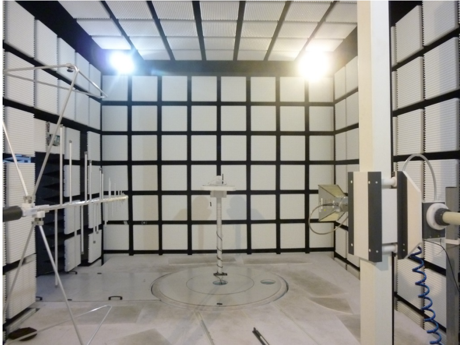
Photo 3: EUT at the anechoic chamber, plastic housing (ex version)
