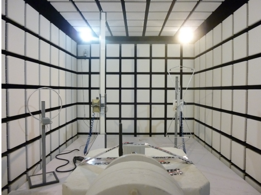
Photo 1: EUT at the anechoic chamber, plastic housing (ex version)
