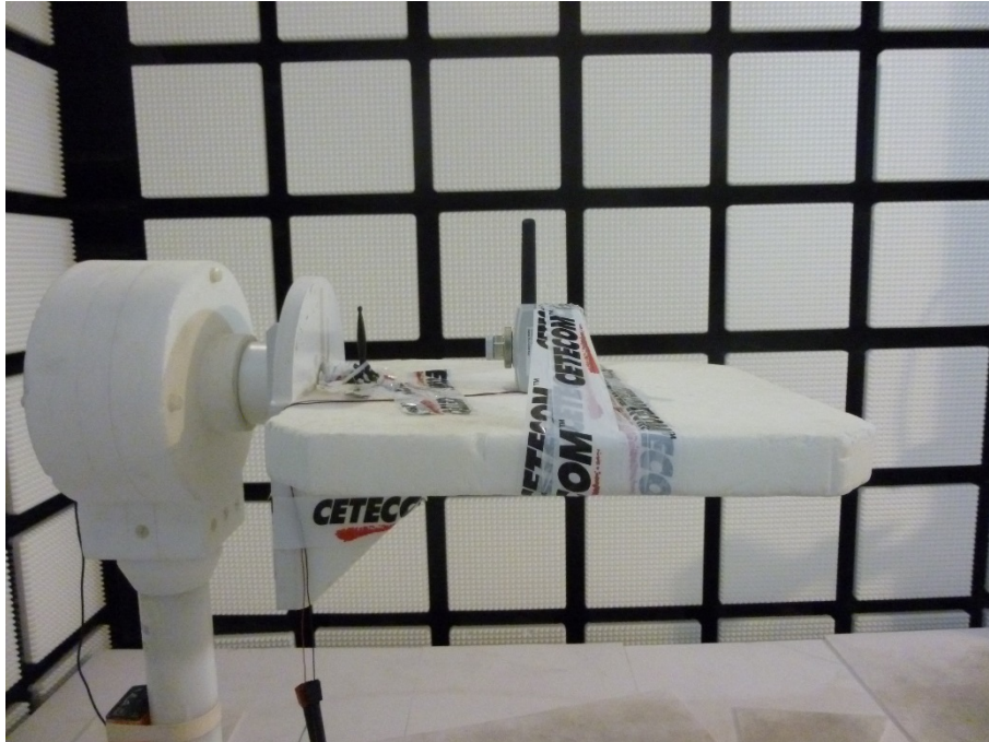
Photo 5: EUT at the anechoic chamber, plastic housing (ex version)
