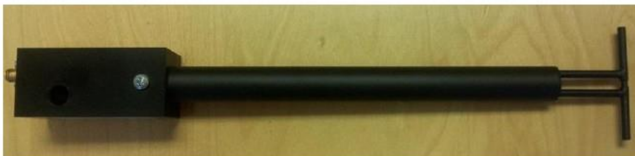
Figure 1 – MVG COMOSAR Validation Dipole
