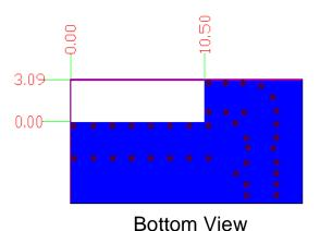
Transmission Line with 50Ω Impedance Characteristic
