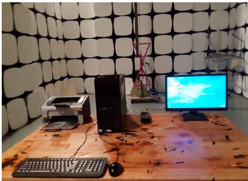
Radiated Emission Test Set-up(30-1000MHz)
