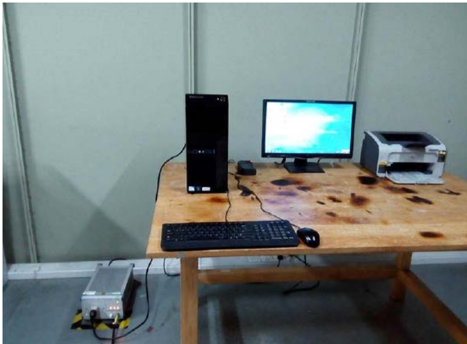
Conducted Emission Test Set-up –Front view
