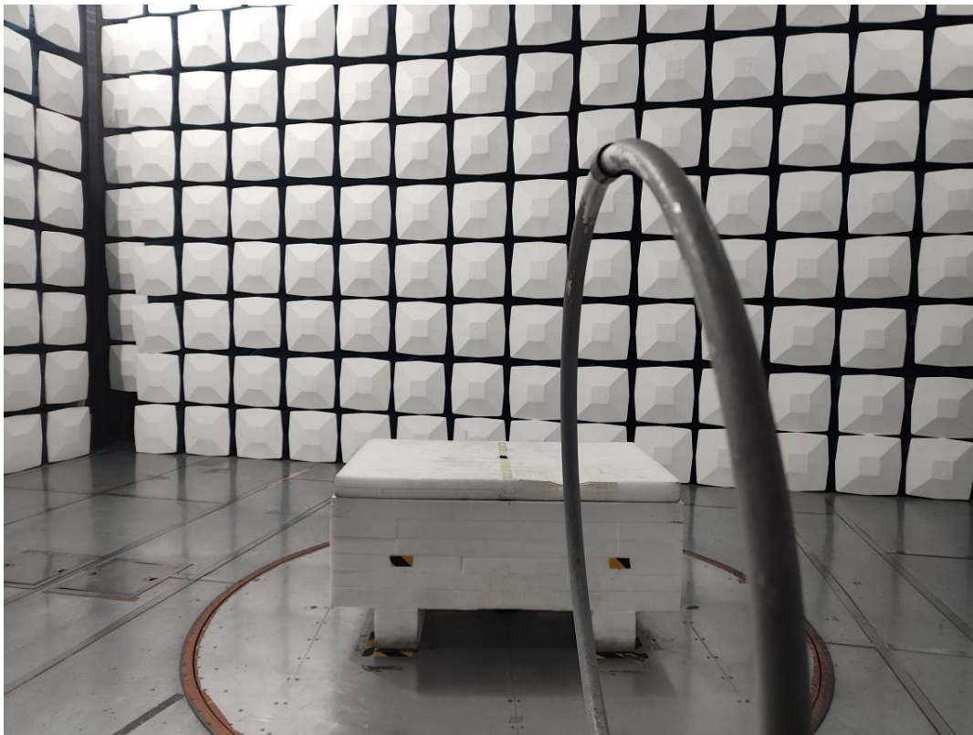
Radiated Emission 9k-30MHz Perpendicular View
