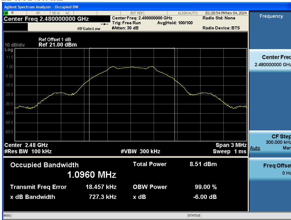
Test Data: BLE 2M\2402MHz
