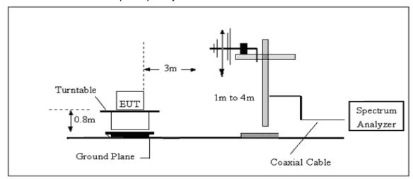
3. Radiated Emission Test-Up Frequency Above 1GHz
