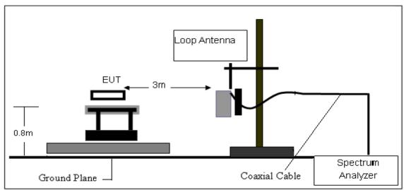
2. Radiated Emission Test-Up Frequency 30MHz~1GHz
