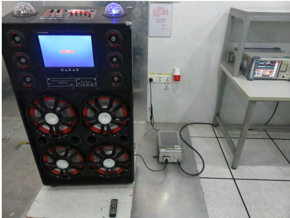
Photo of Conducted Emission Measurement
