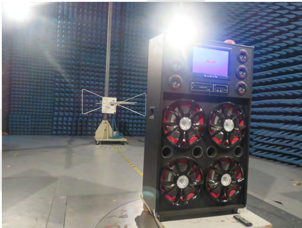
Photo of Radiation Emission Test
