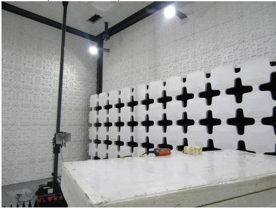
Conducted disturbance voltage at mains ports(150KHz-30MHz)
