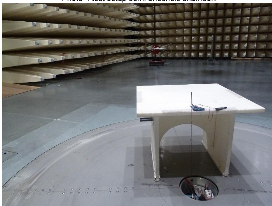
Photo 4 test setup semi anechoic chamber:
