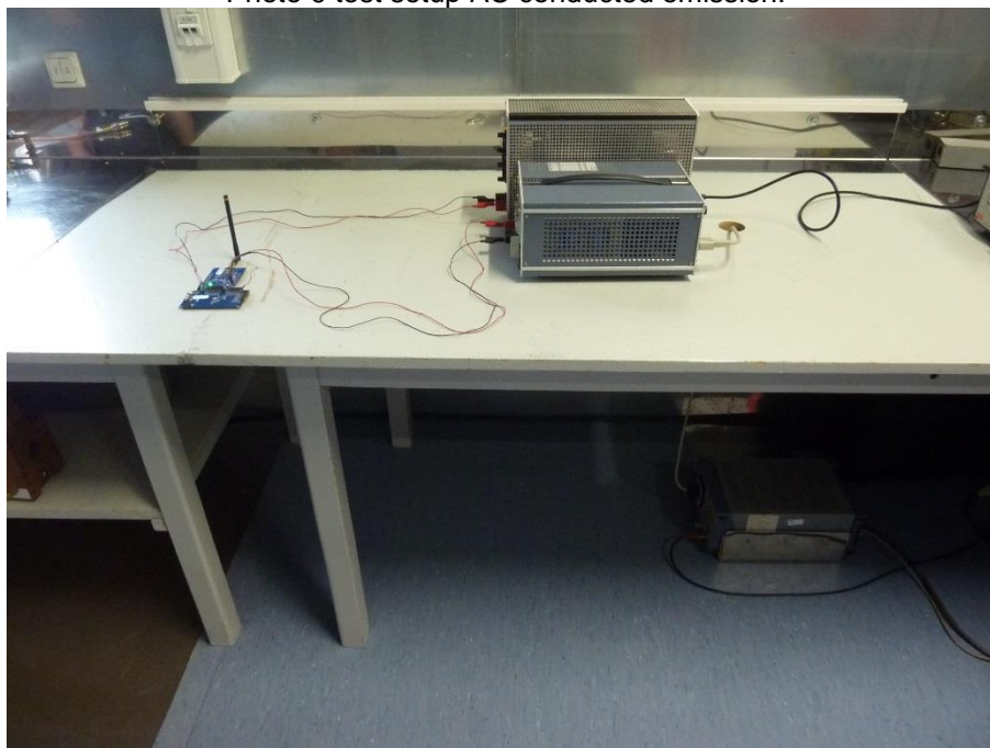
Photo 9 test setup AC conducted emission:
