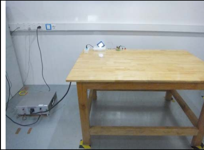
Conducted Emissions Test Setup Front View
