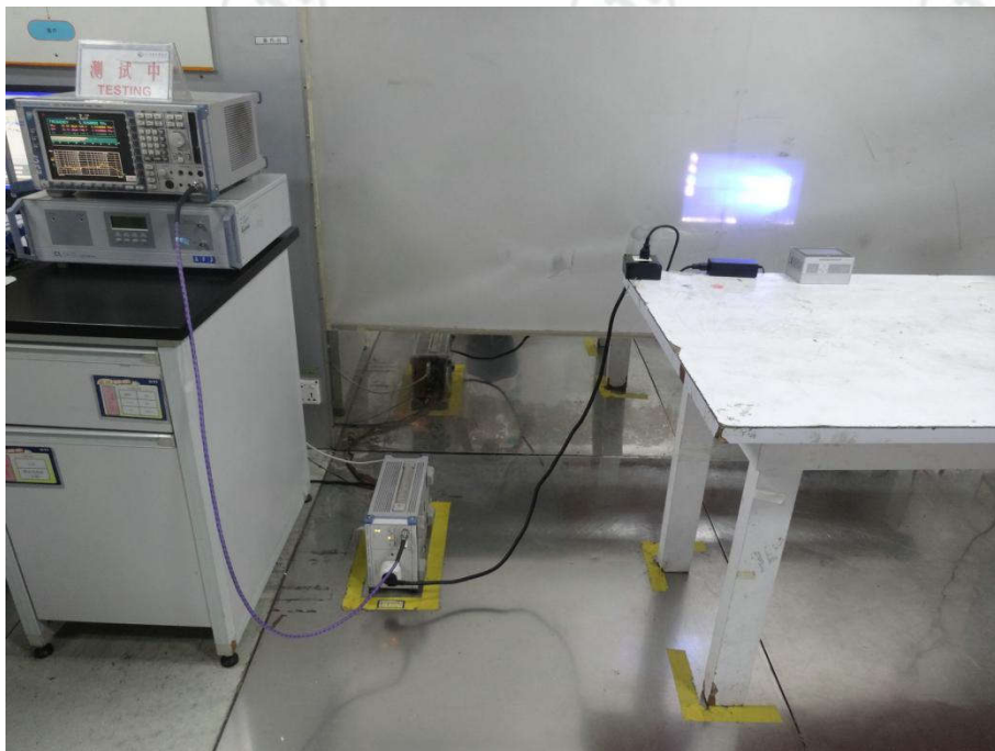
Conducted Emissions Test Setup
