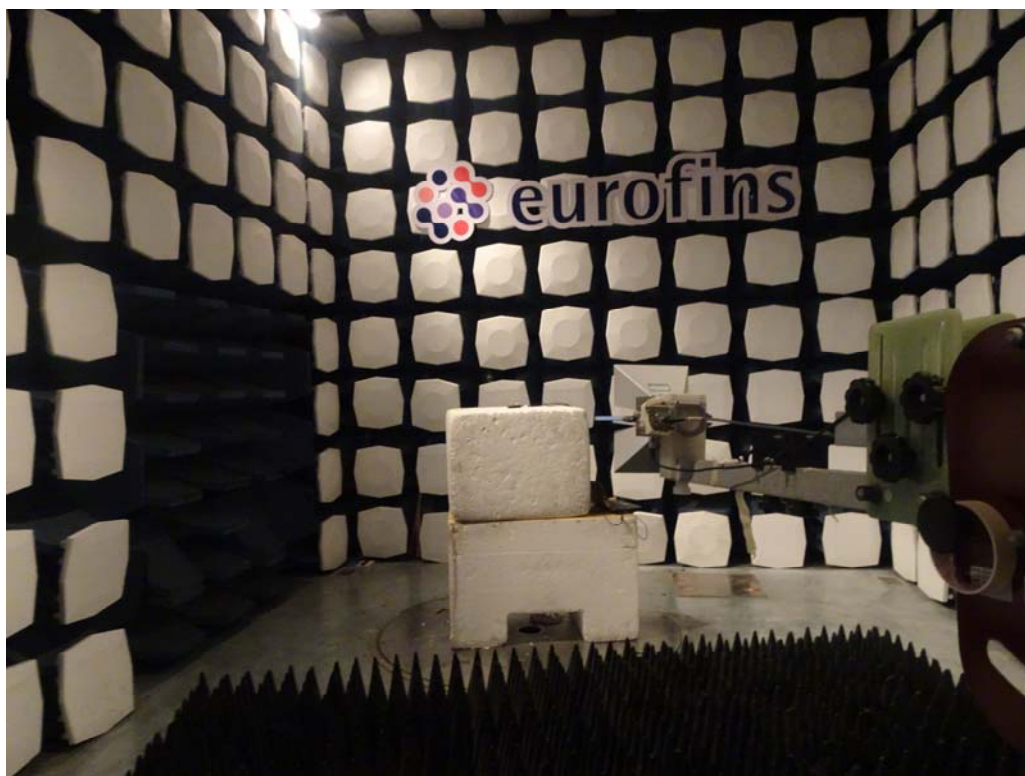
Picture 1 Radiated Emission Test Setup
