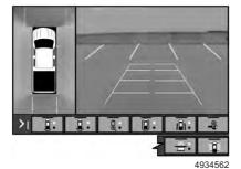
Touch the camera view buttons along the bottom of the infotainment display.
