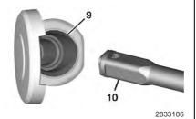
3. Insert the hoist end (open end) (10) of the extension through the hole (9) in the rear bumper.
