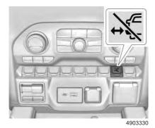
The power assist steps can be extended to the tire by pressing When extending the steps with the kick switch is disabled. The vehicle must be in P (Park) or N (Neutral).
