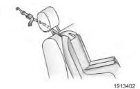
If the position you are using has an adjustable head restraint and you are using a single tether, raise the head restraint and route the tether under the head restraint and in between the head restraint posts.
