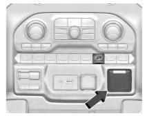
In Cab Power Outlet and DC/AC Switch
