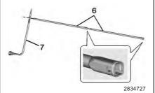
2. Assemble the wheel wrench (7) and the two jack handle extensions (6), as shown.
