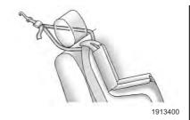
If the position you are using has an adjustable head restraint and you are using a dual tether, route the tether around the head restraint.
