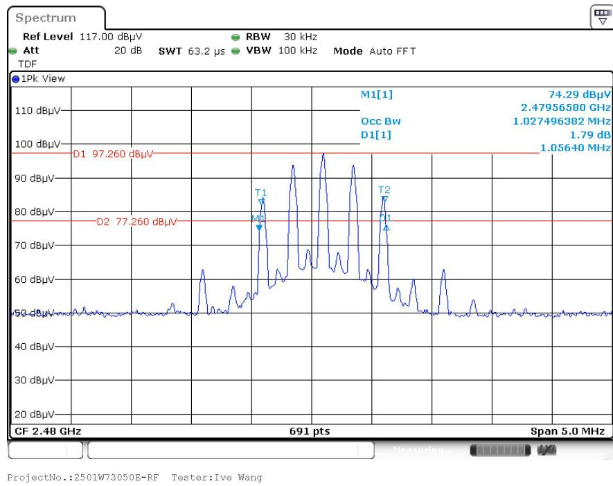
Note: The TDF is the parameter of the Multiplex Switch Test Control Set and does not include the antenna factor, cable loss and amplifier factor.
